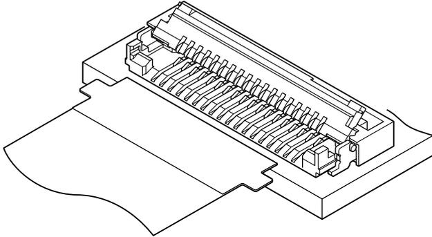
**The connector for the 0.3mm thickness FPC with a mounting height of 1.3mm. FPC with protrusion prevents incomplete insertion and mis-insertion, so that it provides reliable connection.**
