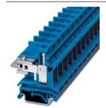
N disconnect terminal block, Special and hybrid connection, Cross section: 0.5 mm² - 16 mm², AWG: 20 - 6, Width: 10.2 mm, Color: blue, Mounting type: NS 35/7,5, NS 35/15, NS 32
