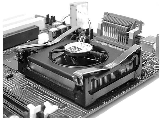
Fig.6 The Usage Example of the Custom Clip
