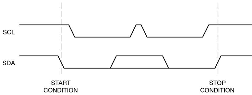
Figure 2. Start/Stop Timing
