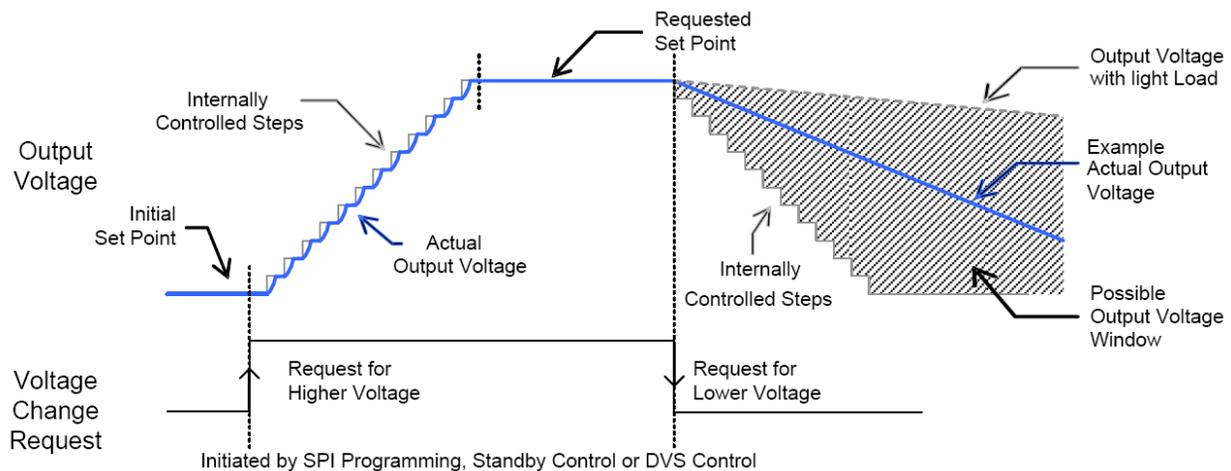
**Figure 20. SW1 Voltage Stepping with Pin Controlled DVS**
