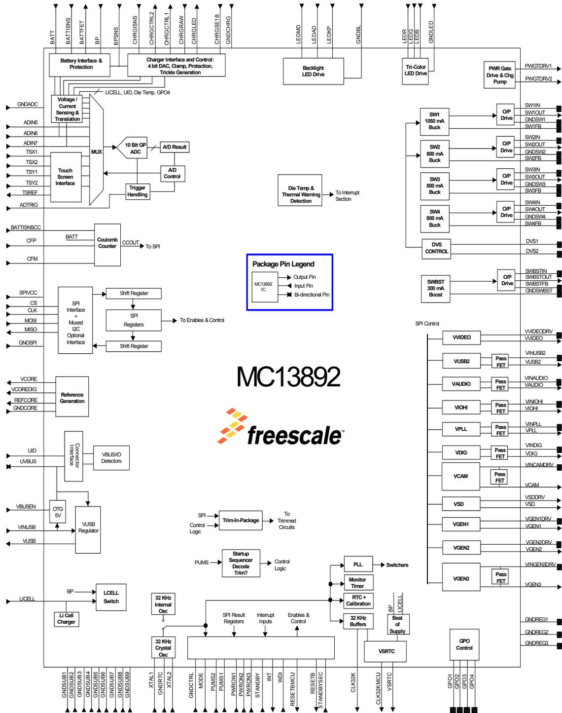
Figure 2. MC13892 Simplified Internal Block Diagram
