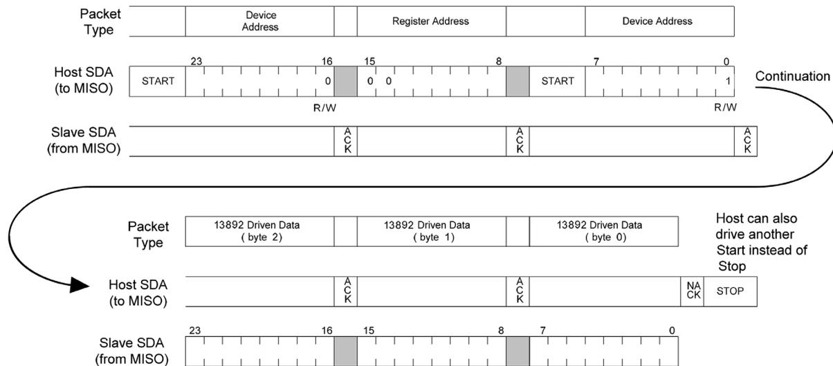
Figure 9. I<sup>2</sup>C 3 Byte Read Example
