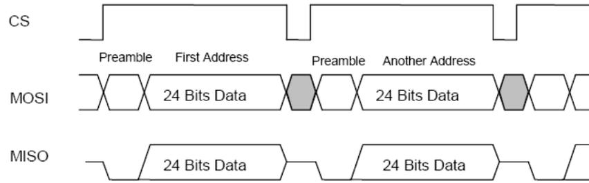
Figure 6. SPI Transfer Protocol Multiple Read/Write Access
