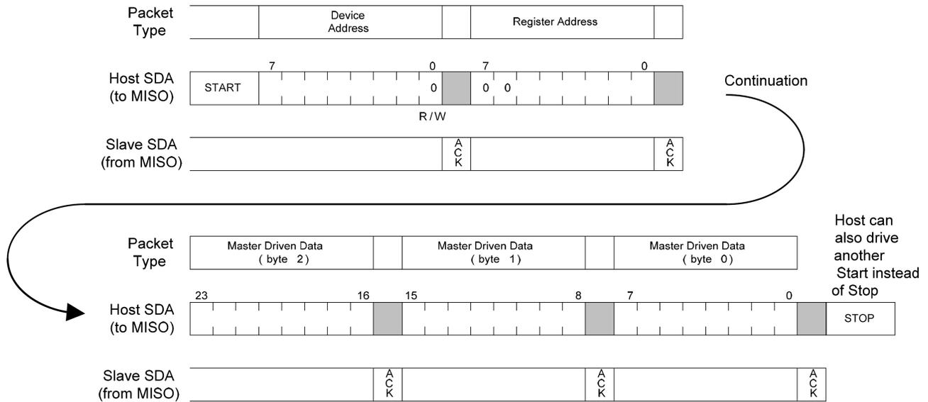
Figure 8. I<sup>2</sup>C 3 Byte Write Example
