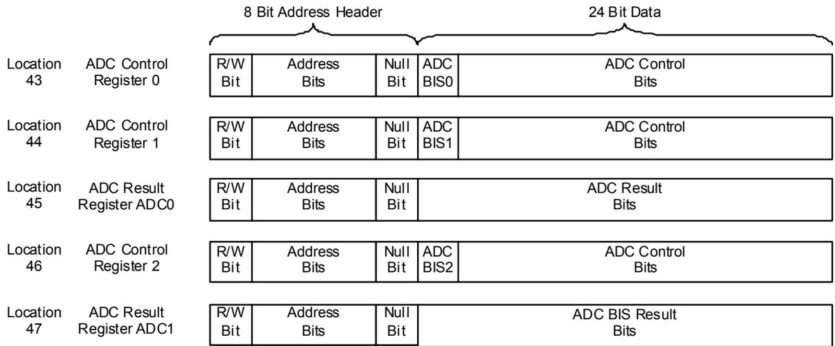
**Figure 28. ADC Register Set for ADC BIS Access**
