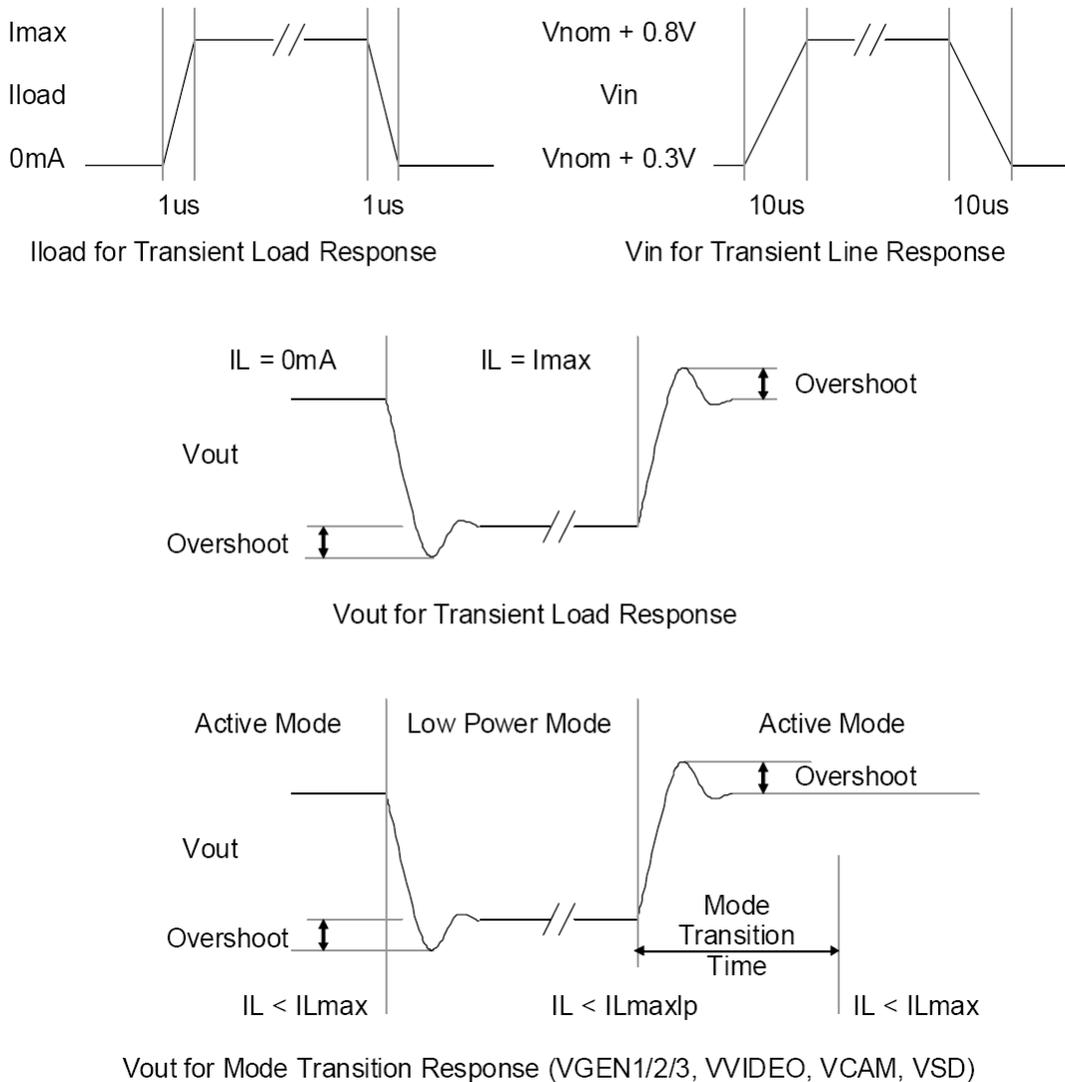
**Figure 25. Transient Waveforms**
