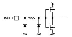
Figure 7. Input Equivalent Circuit
