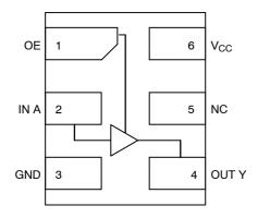
Figure 1. Pinout (Top View)
