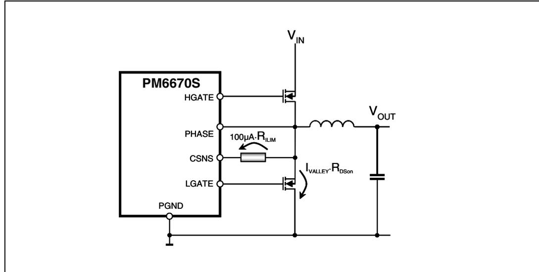
An internal  $120\ \mu\text{A}$  current source is connected to CSNS pin that is also the non-inverting input of the positive current limit comparator. When the voltage drop developed across the sensing parameter equals the voltage drop across the programming resistor  $R_{ILIM}$ , the controller skips subsequent cycles until the overcurrent condition is detected or the output UV protection latches off the device (see [Section 7.1.11: Over voltage and under voltage protections on page 36](#)).
