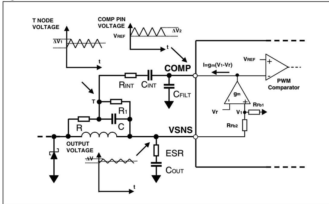
The ripple on the COMP pin is the sum of the output voltage ripple and the triangular ripple generated by the Virtual-ESR network. In fact the Virtual-ESR Network behaves like a another equivalent series resistor  $R_{VESR}$ .
