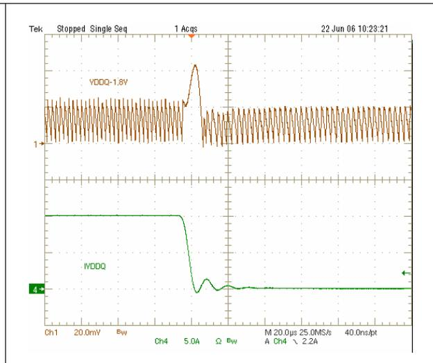
**Figure 23. 0 A to 10 A VDDQ load transient, pulse-skip**
