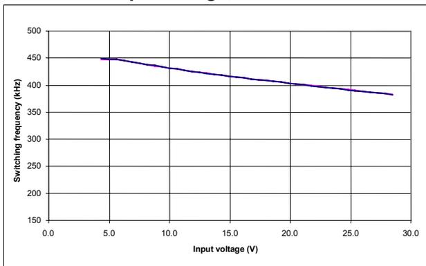
**Figure 6. Switching frequency vs input voltage, 1.5 V**
