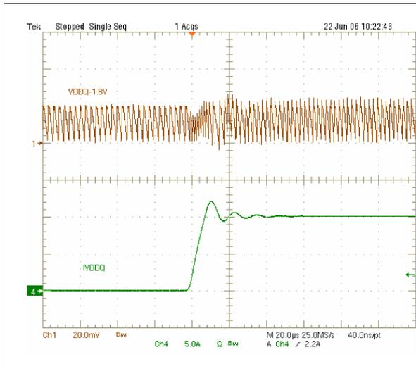
Figure 22. 10 A to 0 A VDDQ load transient, PWM
