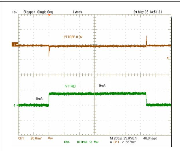
Figure 19. Non-tracking (soft) discharge
