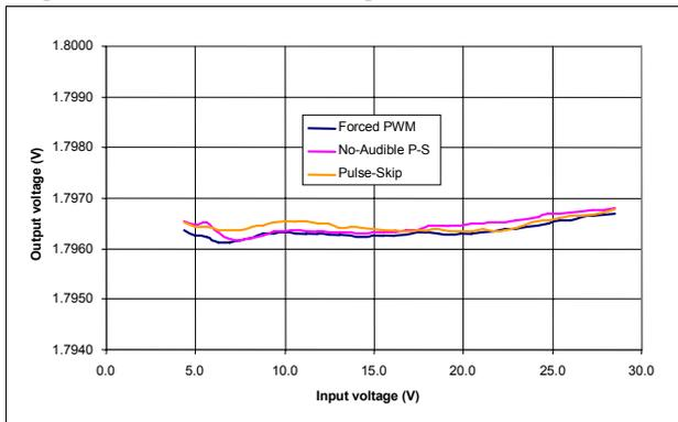
**Figure 8. VDDQ line regulation, 1.5 V, 7 A**
