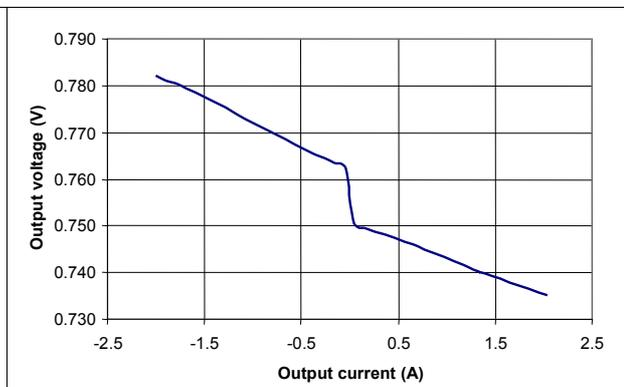
**Figure 13. VTTREF load regulation, 0.9 V,  $VSNS = 1.8 V$**
