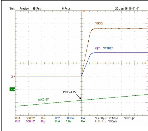
Figure 16. VDDQ soft-start, 1.8 V, heavy load
