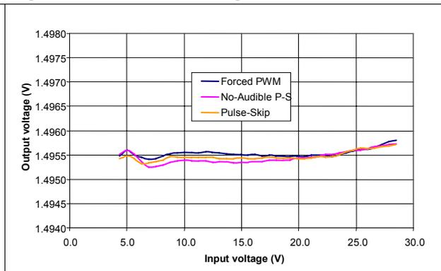
**Figure 9. VDDQ load regulation, 1.8 V,  $V_{IN} = 12 V$**
