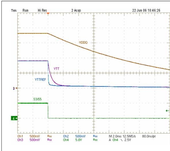
Figure 20. Tracking (fast) discharge, LDOIN = VDDQ
