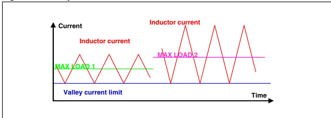
As the valley threshold is fixed, the greater the current ripple, the greater the DC output current will be. If an output current limit greater than  $I_{LOAD(max)}$  over all the input voltage range is required, the minimum current ripple must be considered in the previous formula.
