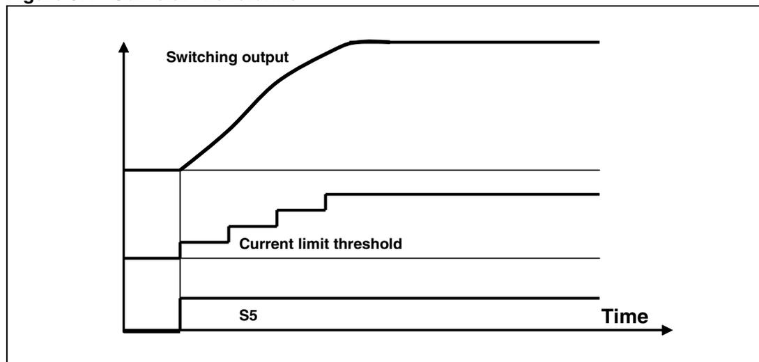
After a fixed 3 ms total time, the soft-start finishes and UVP is released: if the output voltage doesn't reach the under voltage threshold within soft-start duration, the UVP condition is detected and the device performs a soft end and latches off. Depending on the load conditions, the inductor current may or may not reach the nominal value of the current limit during the soft-start (*Figure 38* shows two examples).
