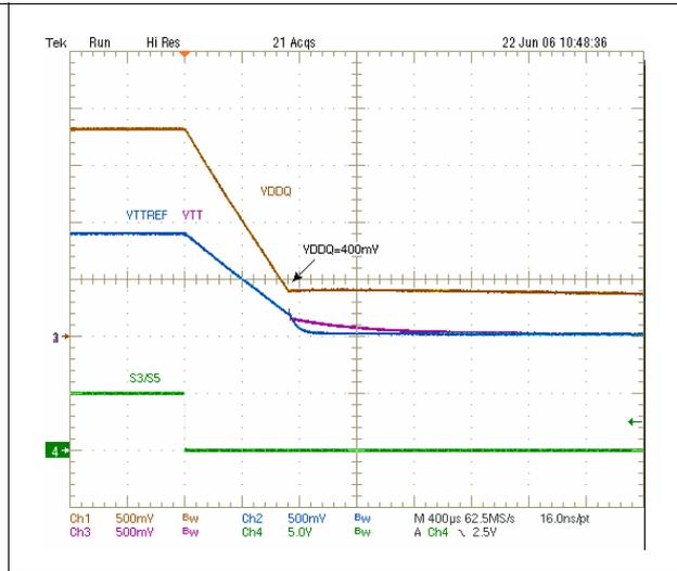
Figure 21. 0 A to 10 A VDDQ load transient, PWM
