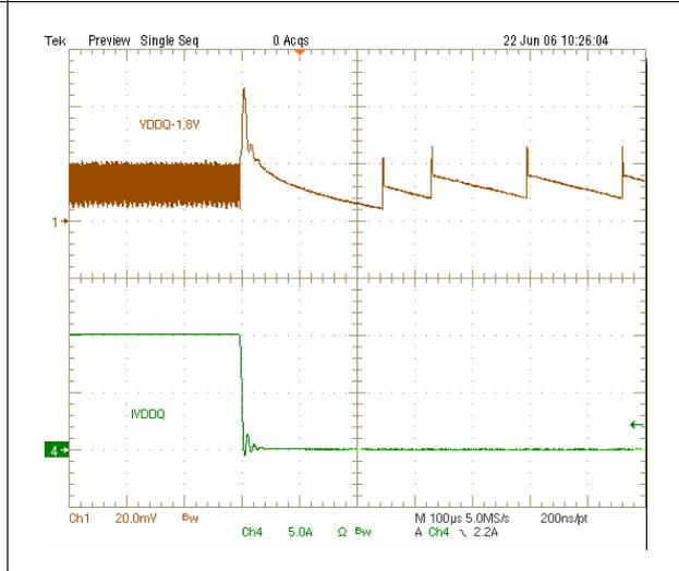
**Figure 25. Over-voltage protection, VDDQ = 1.8 V**
