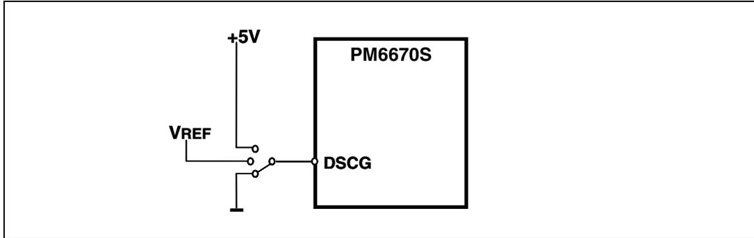
The PM6670S allows the user to choose between fast discharge (tracking discharge), soft discharge (non-tracking discharge) or no discharge modes. Voltage on DSCG multilevel pin determines discharge mode as shown in [Table 9 on page 34](#).
