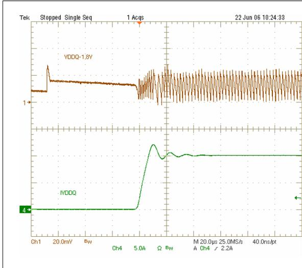
**Figure 24. 10 A to 0 A VDDQ load transient, pulse-skip**
