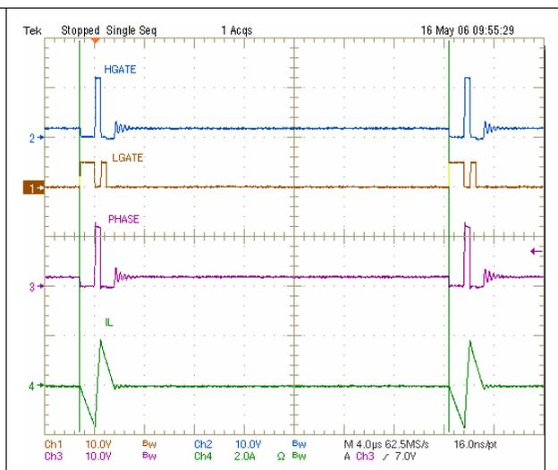
Figure 15. Power-up sequence - AVCC above UVLO
