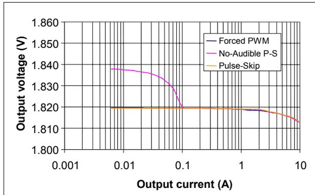
**Figure 10. VDDQ load regulation, 1.5 V,  $V_{IN} = 12 V$**
