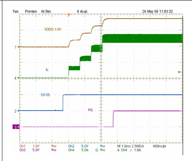
Figure 17. -1.8 A to 1.8 A VTT load transient, 0.9 V
