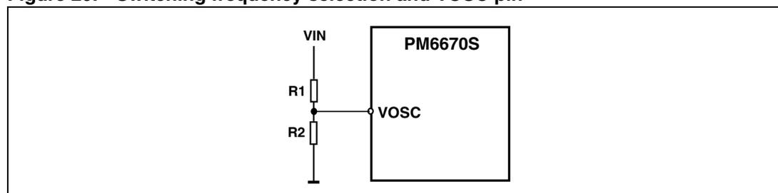
The suggested voltage range for VOSC pin is 0.3 V to 2 V, for better switching frequency programmability.
