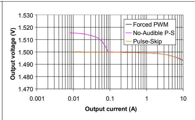
**Figure 11. VTT load regulation, 0.9 V,  $LDO_{IN} = 1.8 V$**
