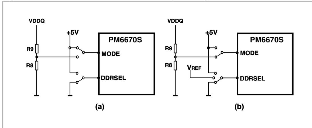
The PM6670S has been designed to satisfy the widest range of applications involving DDR2/3 memories, SSTL15-18 buses termination and I/O supplies for CPU/chipset. The device is provided with multilevel pins which allow the user to choose the appropriate configuration. The MODE pin is used to firstly decide between fixed preset or adjustable (user defined) output voltages.
