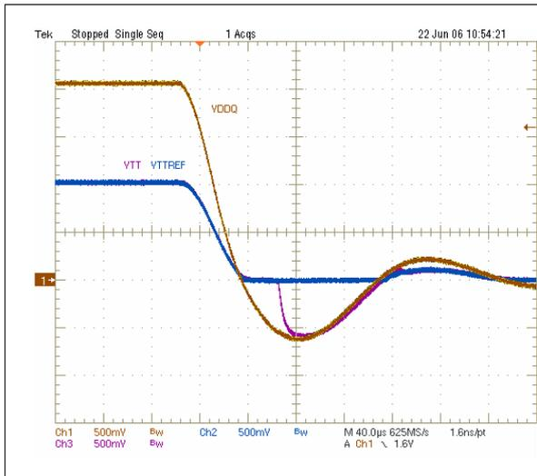
**Figure 26. Under-voltage protection, VDDQ = 1.8 V**
