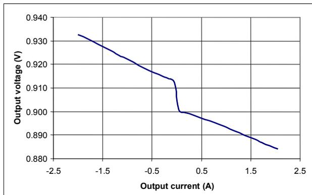
**Figure 12. VTT load regulation, 0.75 V,  $LDO_{IN} = 1.5 V$**
