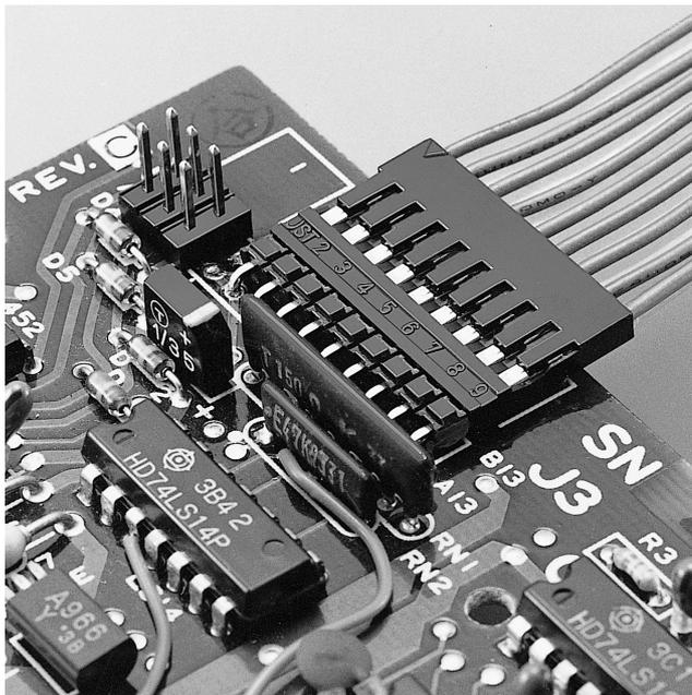
*The RE connector was developed as a highly reliable, low-cost, crimp style connector for connecting wires to printed circuit boards. Well suited for completing the internal connections of office automation equipment, such as personal computers, office computers, and their peripheral devices.*
