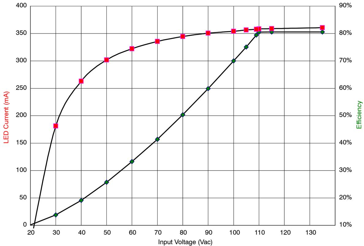
**Figure 6. Line Regulation and Efficiency for 13 W Load**
