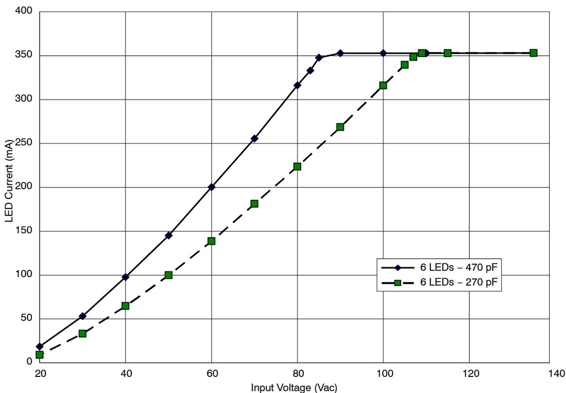
**Figure 9. Line Regulation for 6 LED Load**
