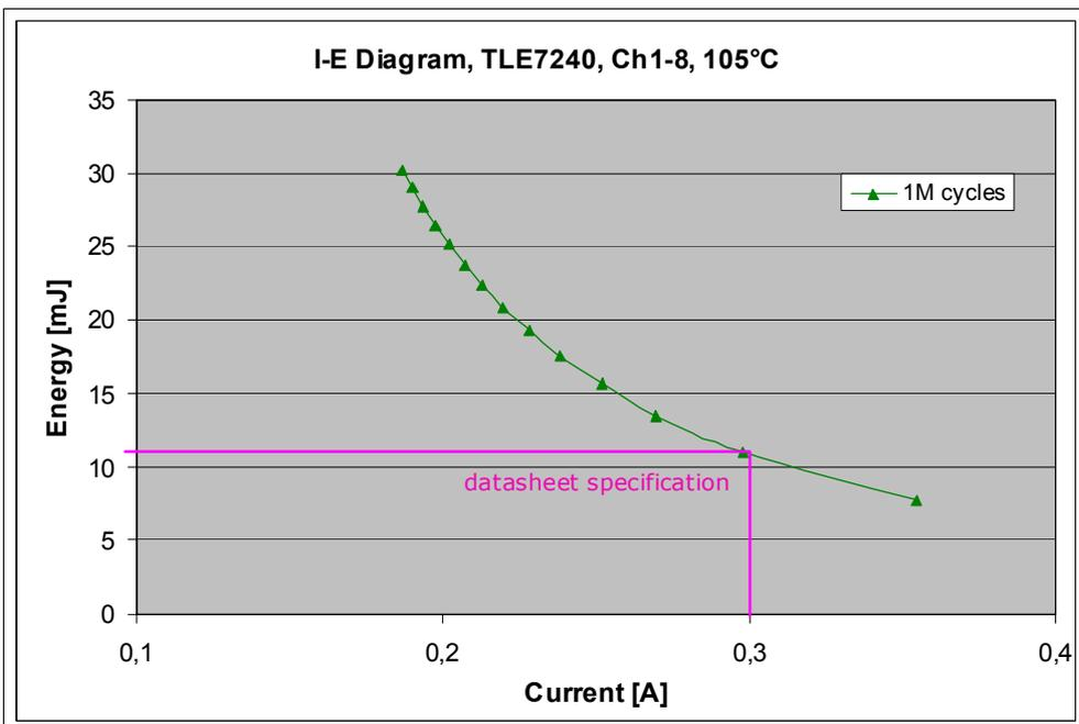
Figure 3 TLE7240SL,  $E_{AR}=f(I_L)$  @ 105°C,  $10^6$  cycles
