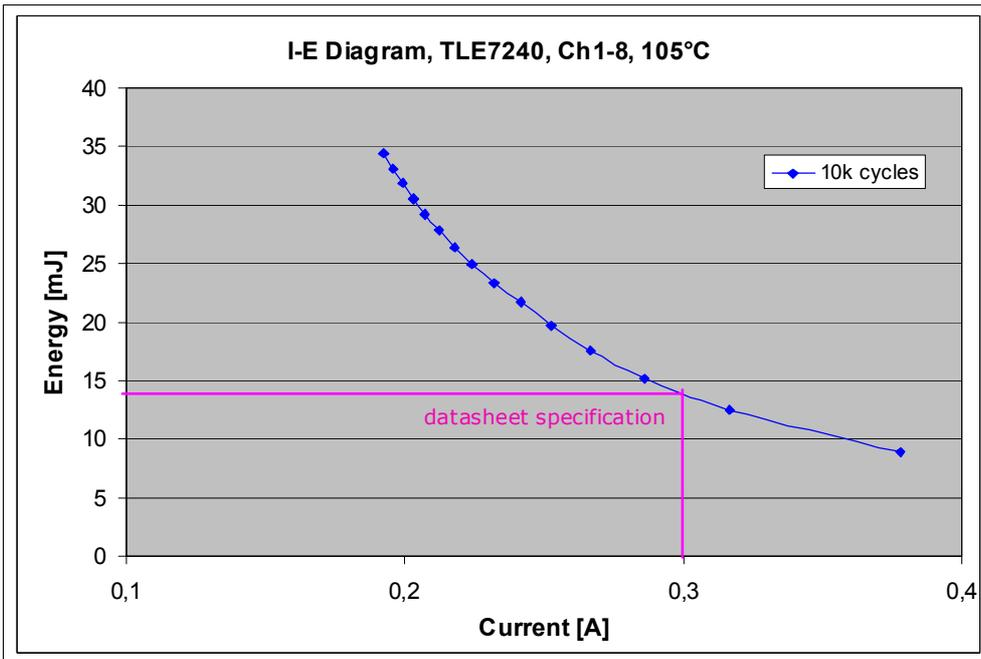
Figure 2 TLE7240SL,  $E_{AR}=f(I_L)$  @ 105°C,  $10^4$  cycles
