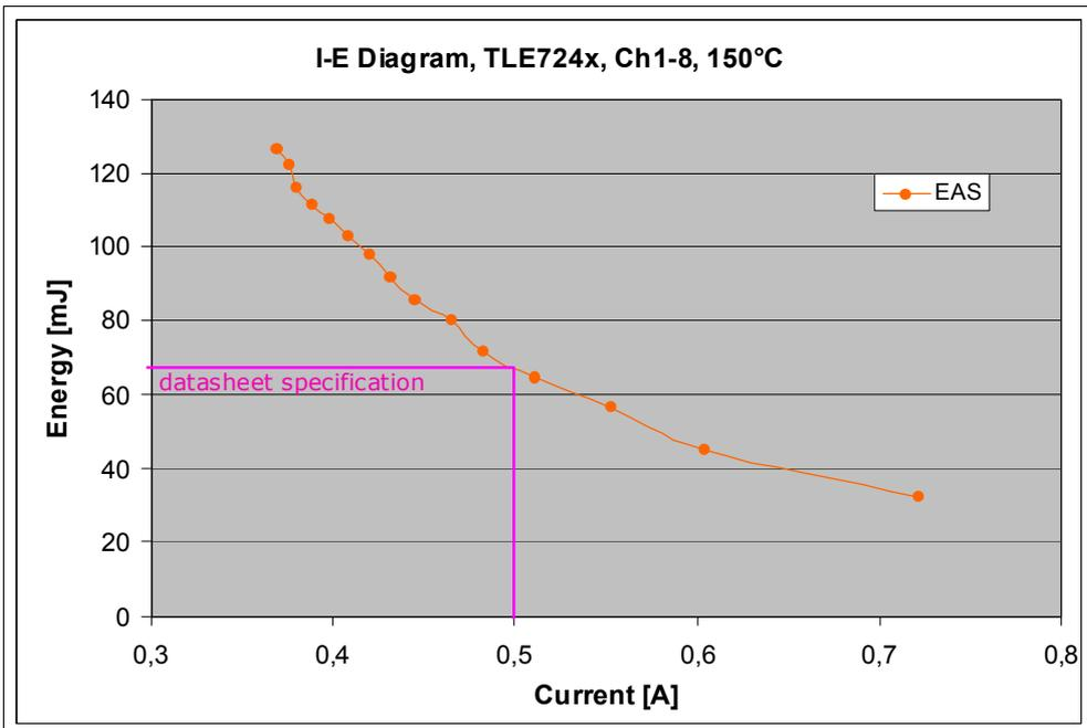
Figure 7 TLE7243SL, TLE7244SL,  $E_{AS}=f(I_L)$  @ 150°C
