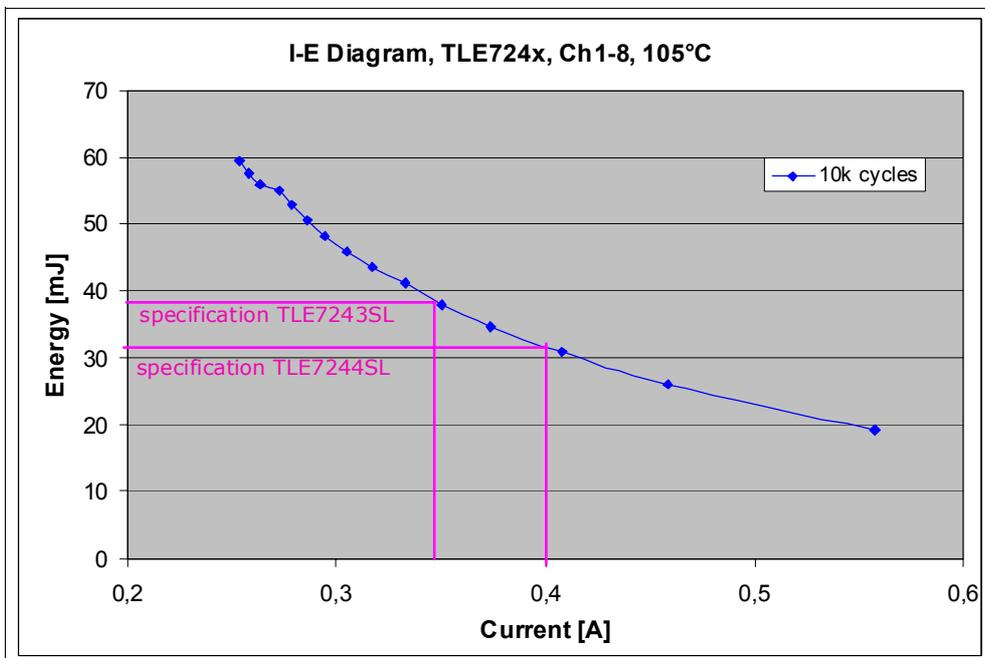
Figure 5 TLE7243SL, TLE7244SL,  $E_{AR}=f(I_L)$  @ 105°C,  $10^4$  cycles
