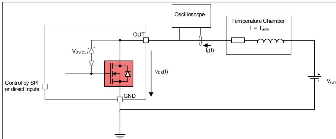
**Figure 8**  $E_A$  measurement setup
