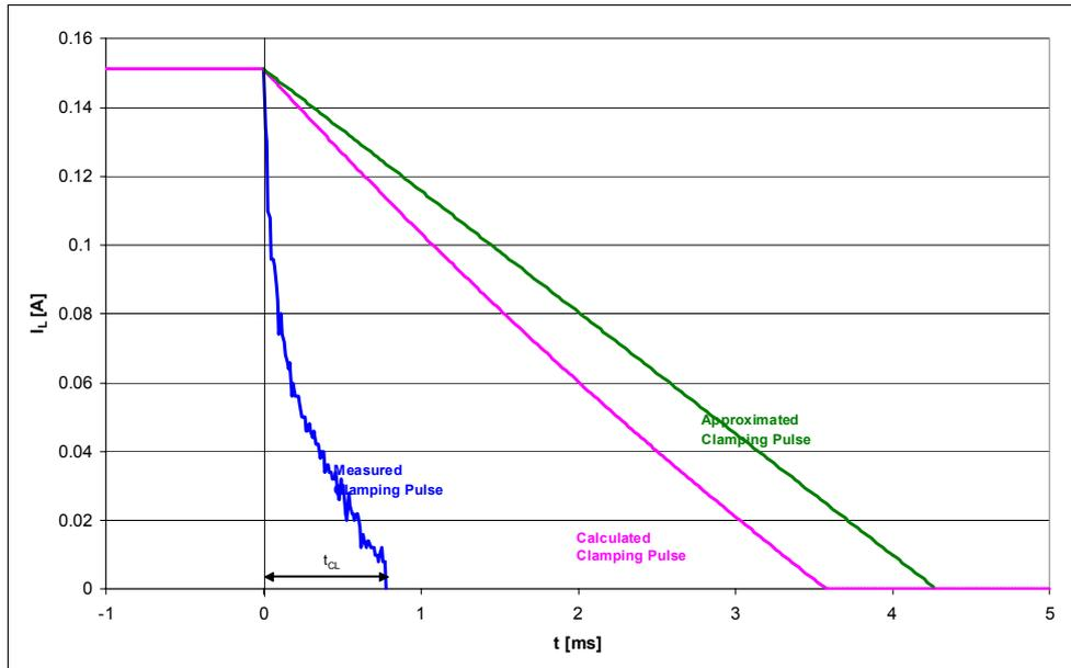
**Figure 9**  $E_A$  measurement ( $R_L=89.3\Omega$ ,  $L_L=920\text{mH}$ ,  $V_{BAT}=13.5\text{V}$ )
