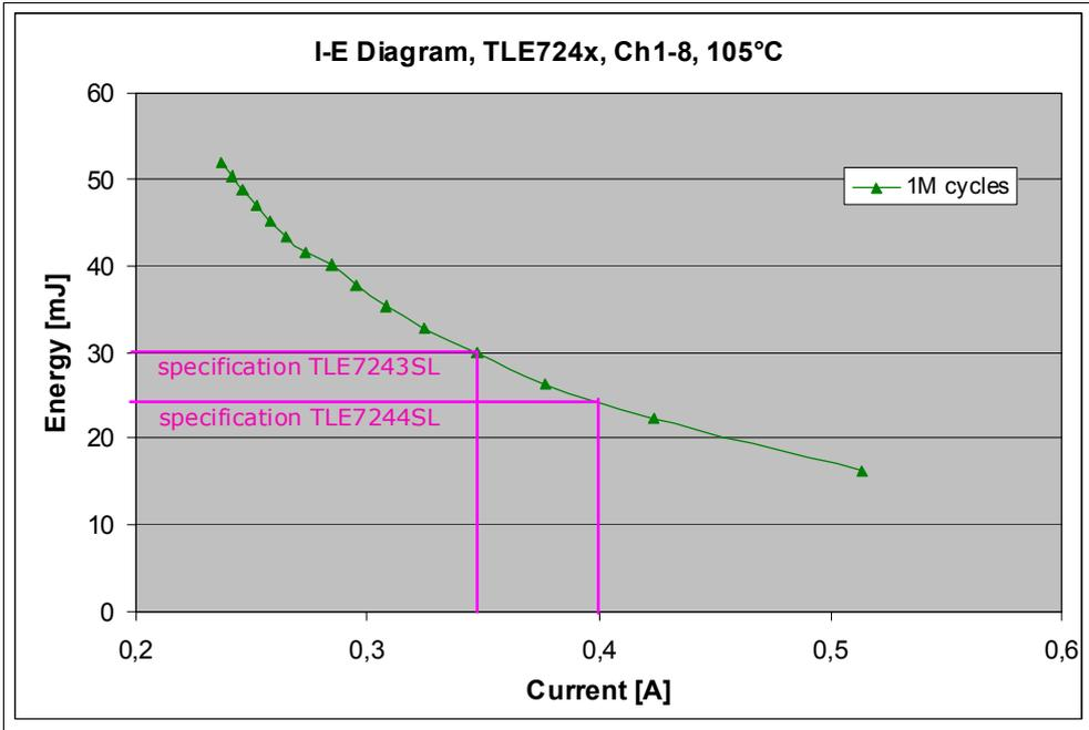
Figure 6 TLE7243SL, TLE7244SL,  $E_{AR}=f(I_L)$  @ 105°C,  $10^6$  cycles
