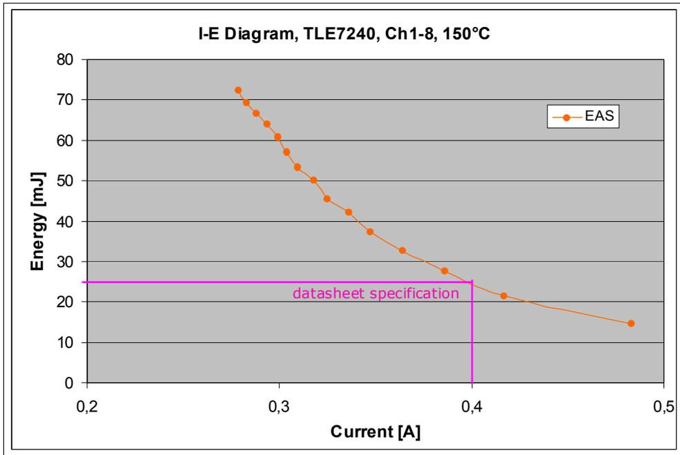
Figure 4 TLE7240SL,  $E_{AS}=f(I_L)$  @ 150°C
