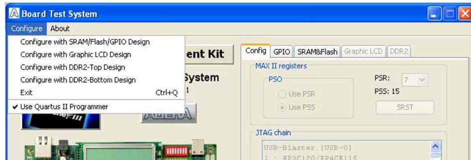
1. To configure the FPGA with a test system design, perform the following steps: On the Configure menu, click the configure command that corresponds to the functionality you wish to test.
