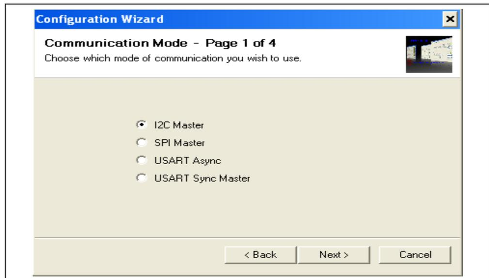
**FIGURE 1-4:** Step 1 - Communication Mode Selection.
