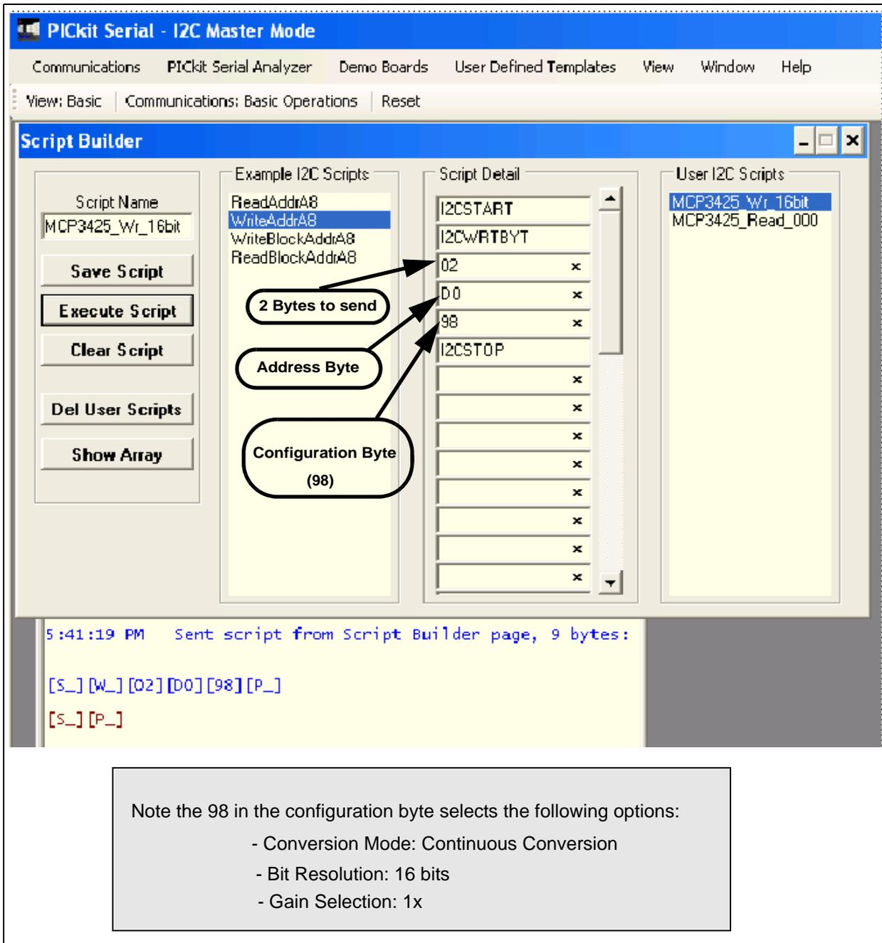
**FIGURE 1-11:** Script File Example for the I<sup>2</sup>C Write Command.
