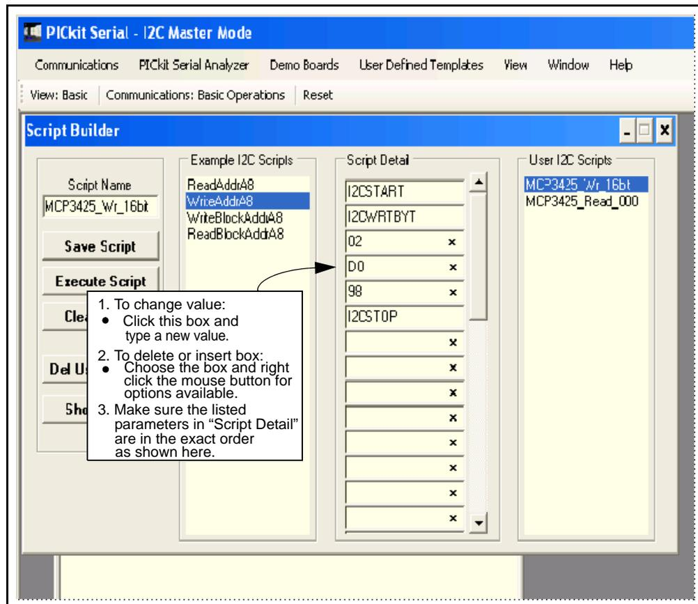
**FIGURE 1-10:** Modifying Parameters in the Script Builder Window.
