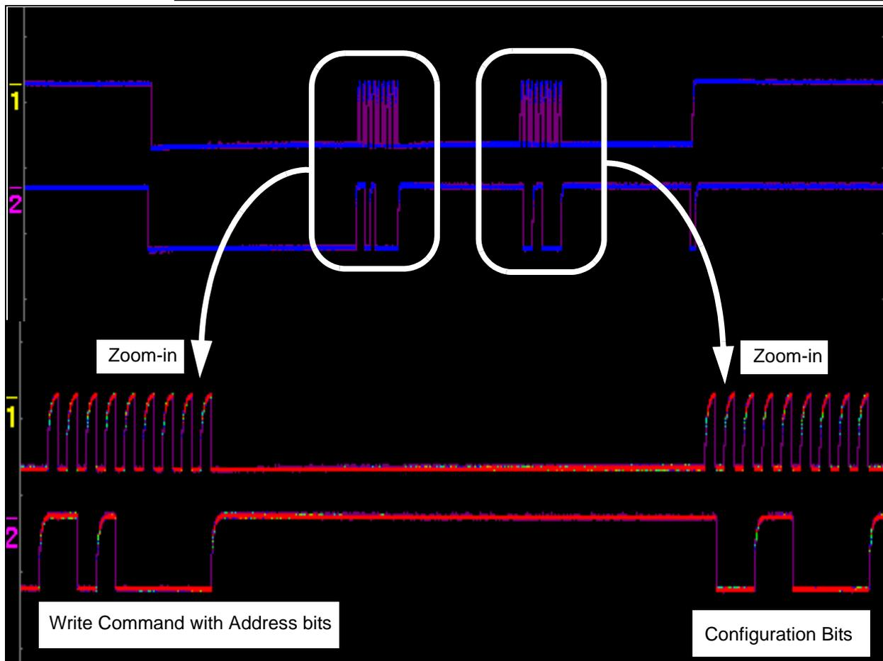
**FIGURE 1-12:** I<sup>2</sup>C Write Command Waveforms for the MCP3425.
