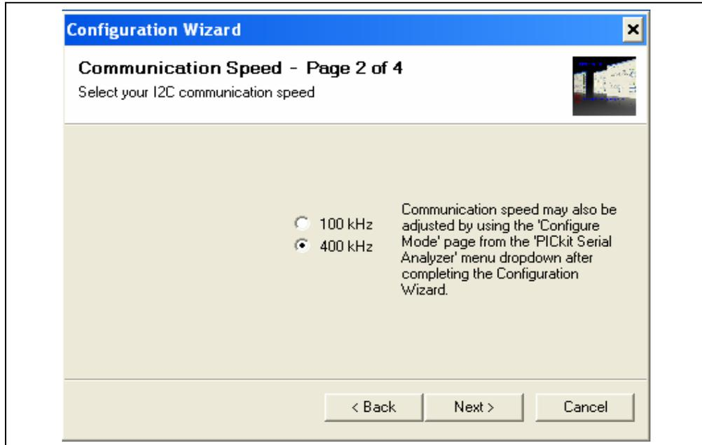
**FIGURE 1-5:** Step 2 - I<sup>2</sup>C Communication Speed Window.
