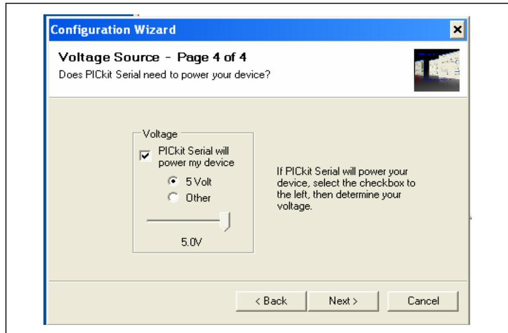
**FIGURE 1-7:** Step 4 - Voltage Source Selection Window.
