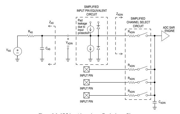
Figure 3-8. ADC Input Impedance Equivalency Diagram
