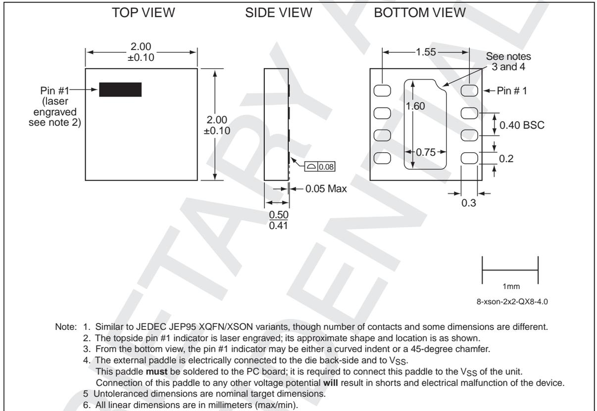
**Figure 12:** 8-Contact Extremely-thin Small Outline No-lead (XSON)
