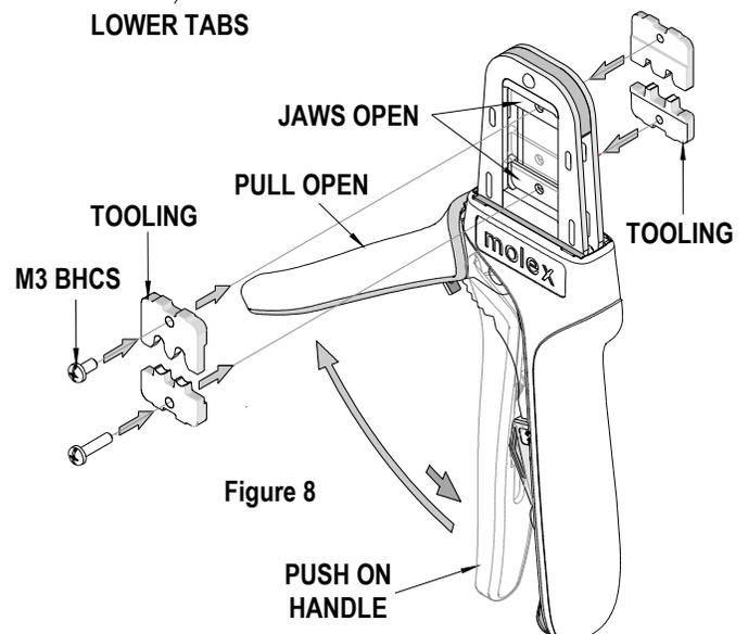
2. Remove the M3 BHCS which is holding the upper tooling.
