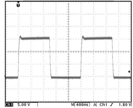
Figure 10 - IXDD414 Typical Waveform F=500KHz, CL=10000pF
