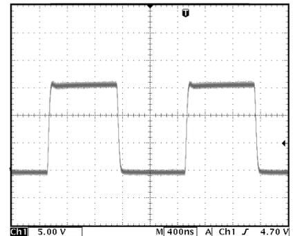
Figure 7 - IXDD408 Typical Waveform F=500KHz, CL=10000pF
