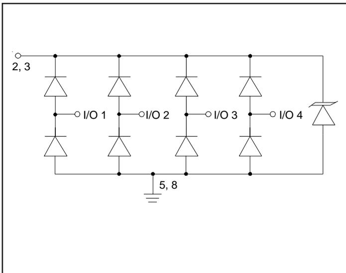
**Schematic and PIN Configuration**
