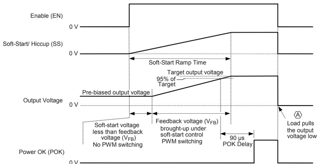
Figure 3: Operation of the Soft-Start Function with Pre-Biasing
