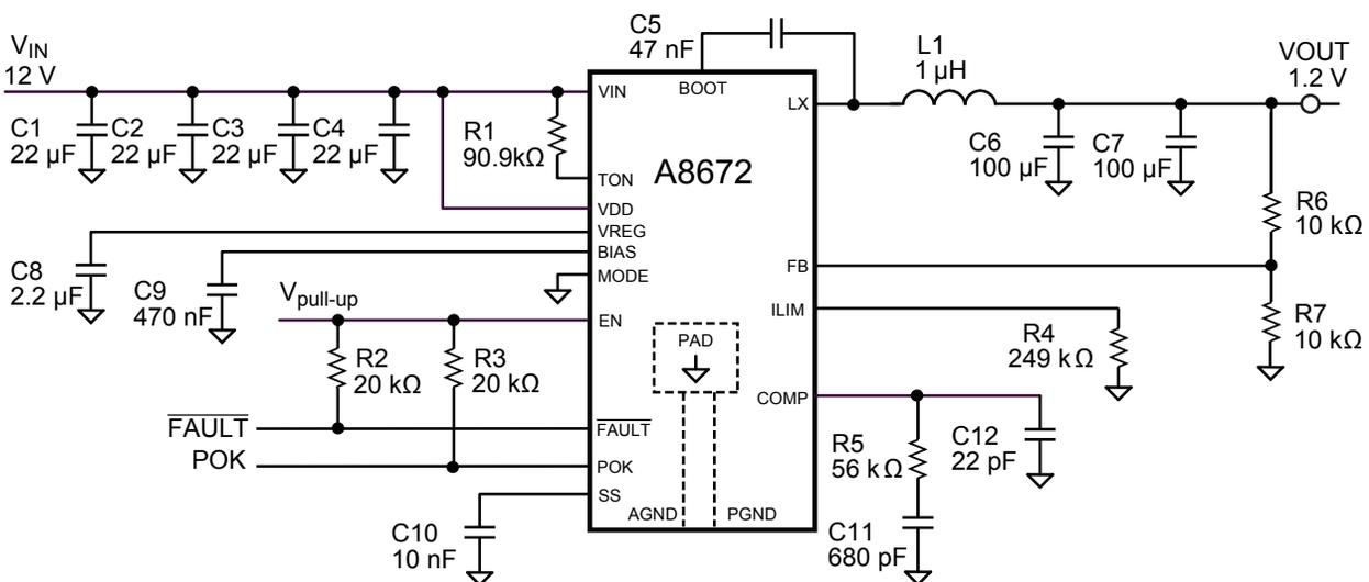
$V_{IN} = 12\text{ V}$ ,  $V_{OUT} = 1.2\text{ V}$ , and  $f_{SW} = 500\text{ kHz}$
