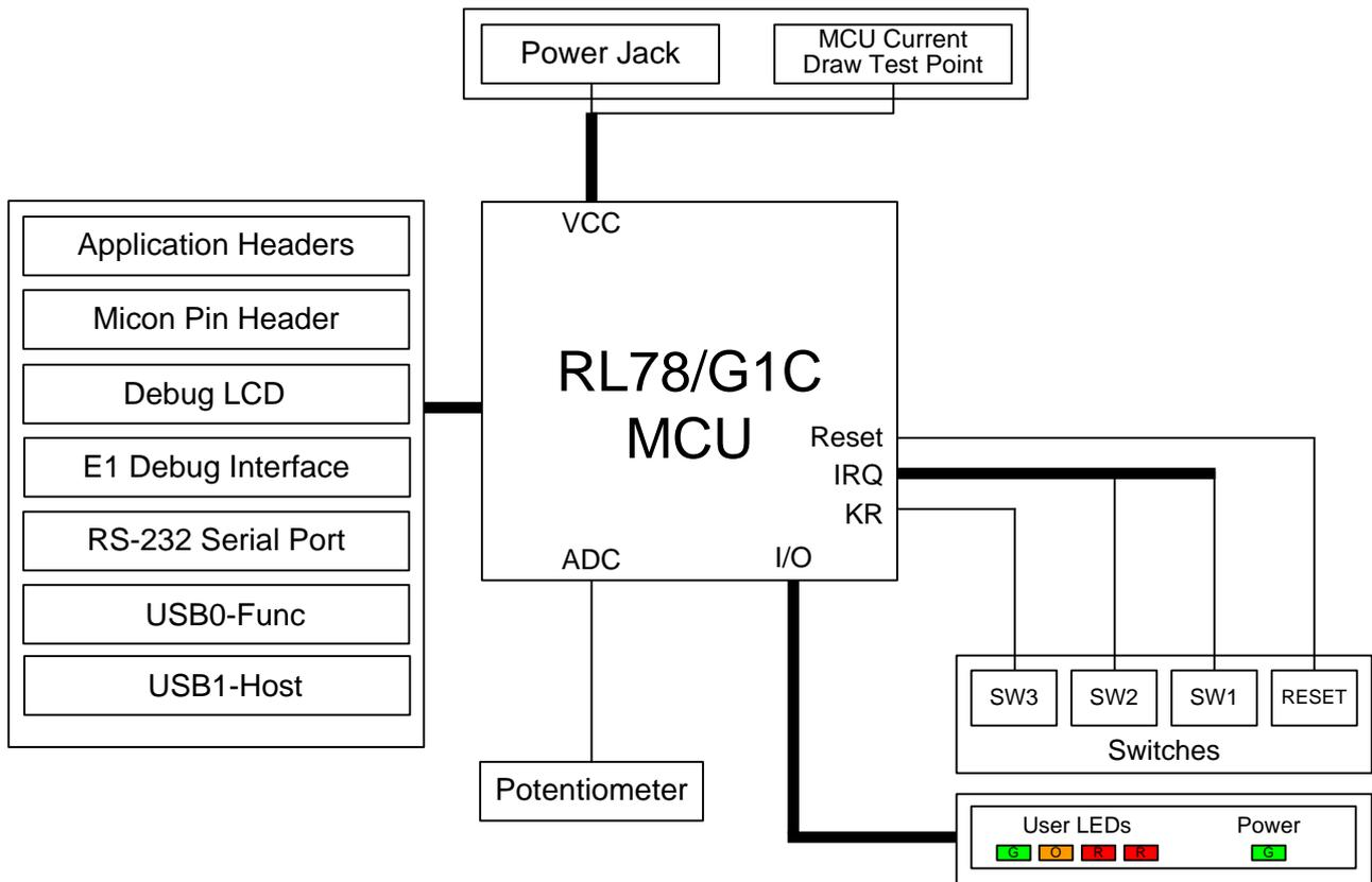
Figure 4-1: Internal RSK Block Diagram
