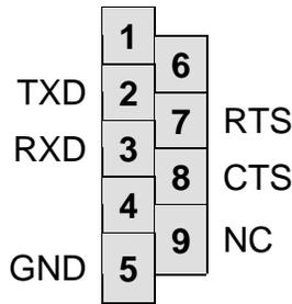
Female DB9 connector that interfaces to the MPU serial port via the U2 RS232 transceiver. It provides simple 2 wire asynchronous serial communications without flow control. Flow control is provided at test points on the module.
