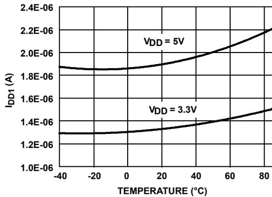
FIGURE 3. I<sub>DD1</sub> vs TEMPERATURE
