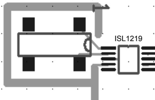
FIGURE 22. SUGGESTED LAYOUT FOR ISL1219 AND CRYSTAL
