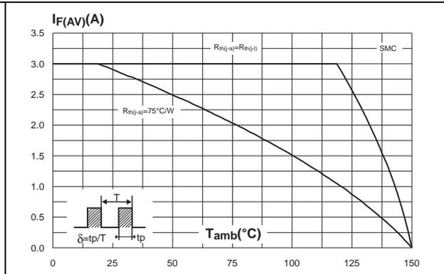
Figure 3. Average forward current versus ambient temperature ( $\delta = 0.5$ ) SMBflat
