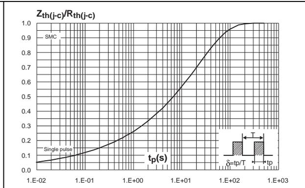
Figure 9. Relative variation of thermal impedance junction to lead versus pulse duration - SMBflat
