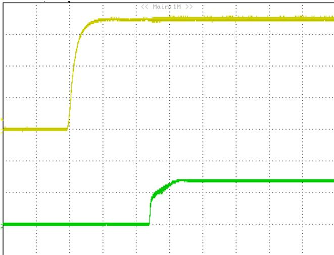
**Figure 11:** Turn on delay time at 7Vin, 0.69V/20A out.
