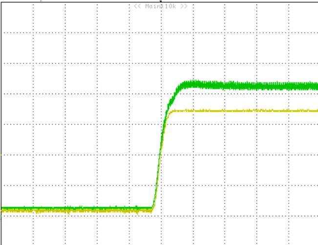
**Figure 25:** Tracking function,  $V_{tracking}=0.8V$ ,  $V_{out}=0.69V$ , full load
