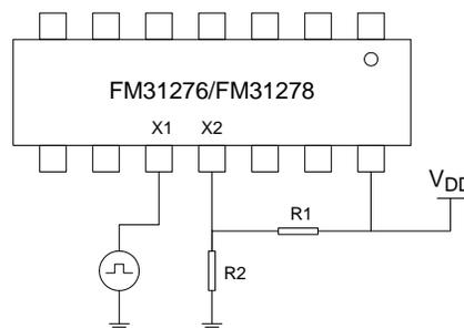
In the example, R1 and R2 are chosen such that the X2 voltage is centered around the X1 oscillator drive levels. If you wish to avoid the DC current, you may choose to drive X1 with an external clock and X2 with an inverted clock using a CMOS inverter.
