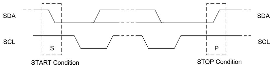
Figure 13. Data Transfer on the I<sup>2</sup>C Bus
