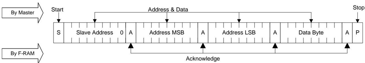
Figure 18. Multi-Byte Write
