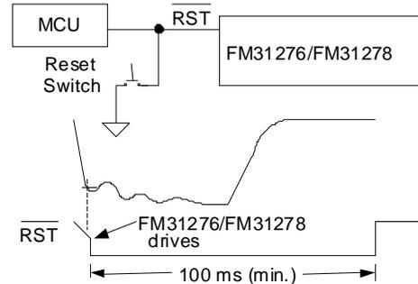
Note The internal weak pull-up eliminates the need for additional external components.
