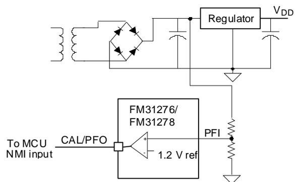
The voltage on the PFI input pin is compared to an onboard 1.2 V reference. When the PFI input voltage drops below this threshold, the comparator will drive the CAL/PFO pin to a ILOW state. The comparator has 100 mV (max) of hysteresis to reduce noise sensitivity, only for a rising PFI signal. For a falling PFI edge, there is no hysteresis.
