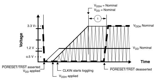
Figure 2-3. Start-Up Sequence with  $V_{DD}$  Raised Before  $V_{DDH}$  with CLKIN Started with  $V_{DDH}$
