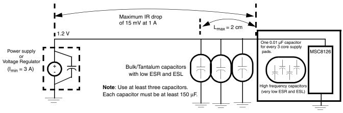
Figure 4-1. Core Power Supply Decoupling
