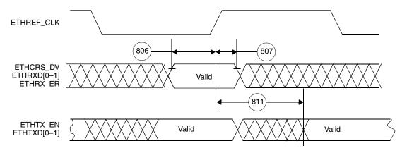
Figure 2-20. RMII Mode Signal Timing
