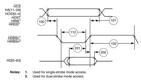
Figure 2-11. Asynchronous Broadcast Write Timing Diagram
