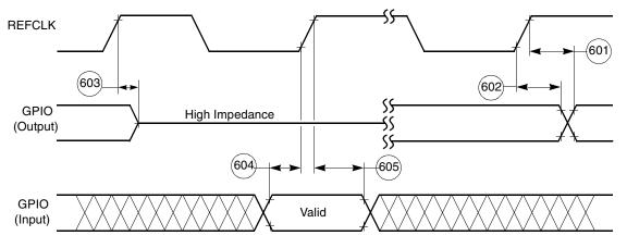
Figure 2-22. GPIO Timing
