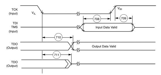
Figure 2-26. Test Access Port Timing Diagram
