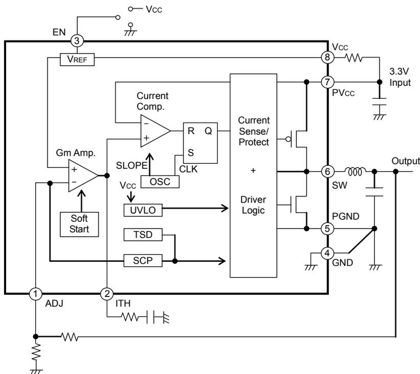
Fig.3 Block Diagram
