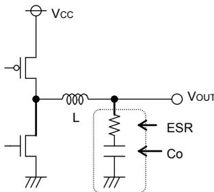
Fig.29 Output capacitor
