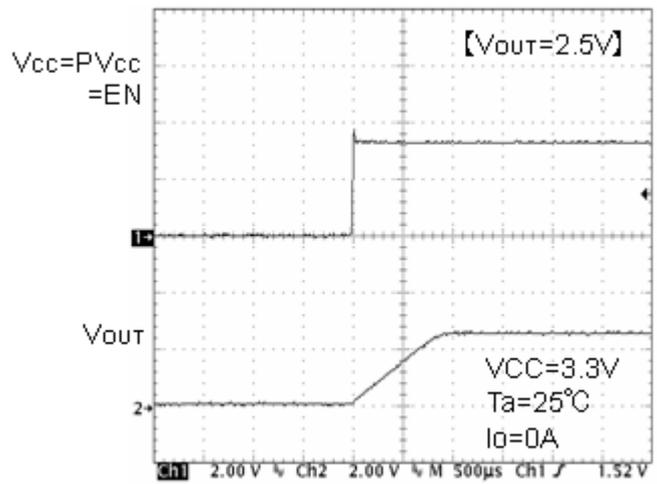
Fig.13 Soft start waveform
