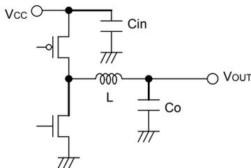
Fig.30 Input capacitor
