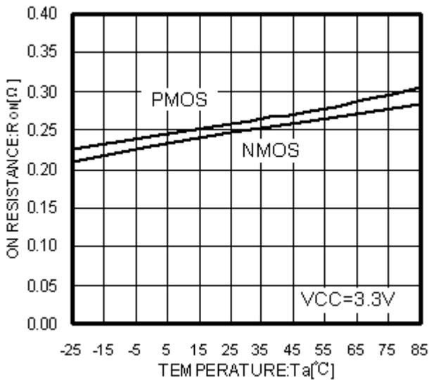
Fig.10 Ta- $R_{on}$
