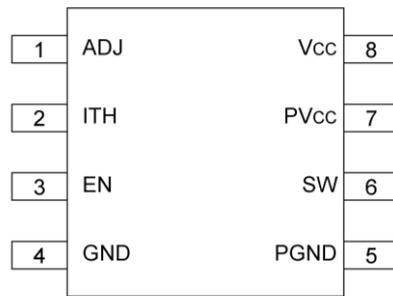
Fig.2 Pin Configuration
