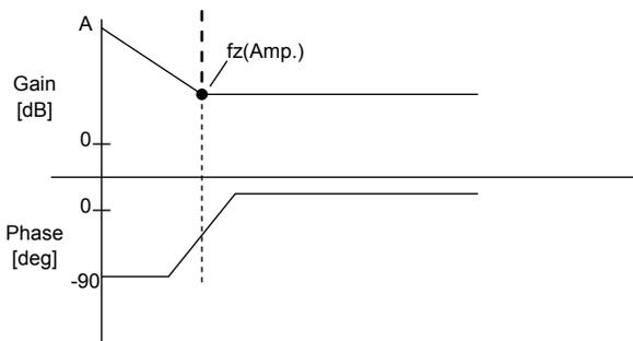
Fig.32 Error amp phase compensation characteristics
