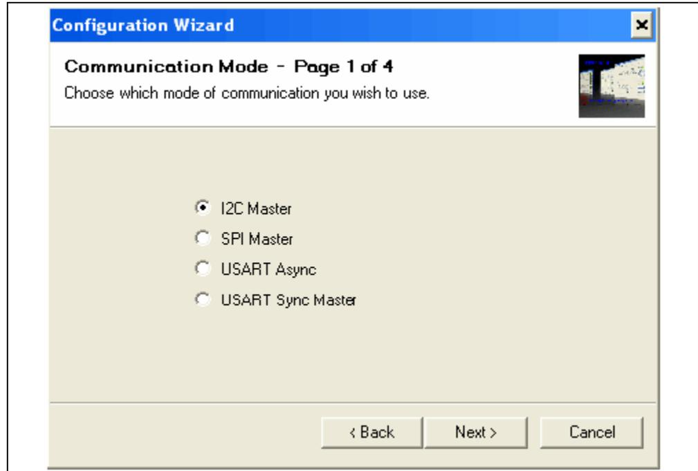
**FIGURE 1-4:** Step 1 - Communication Mode Selection.
