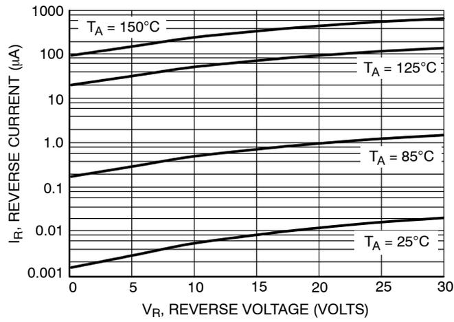
**Figure 3. Leakage Current**
