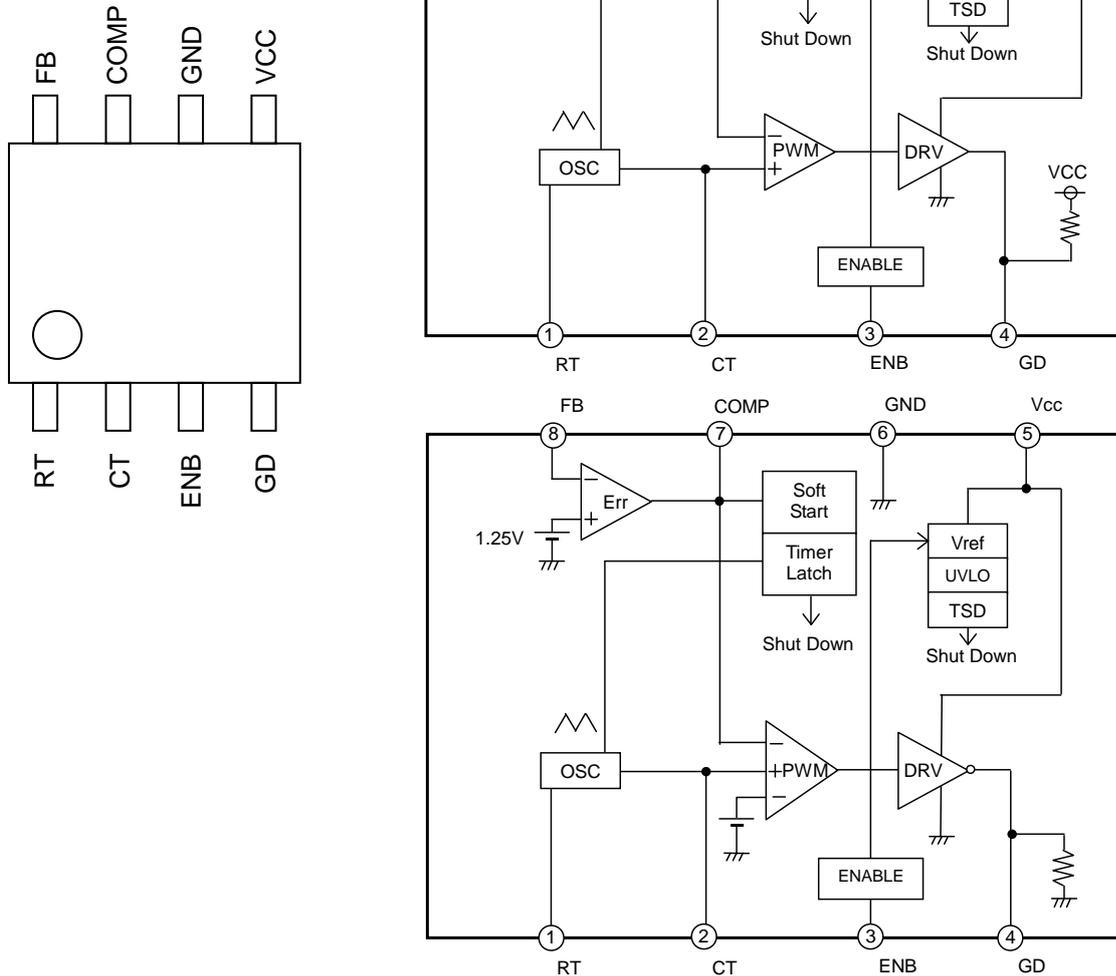
Fig19. Pin Assignment Diagram & Block Diagram (Above:BD9305AFVM / Below:BD9306AFVM)
