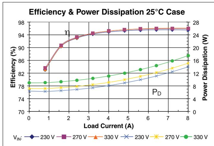
Figure 6 – Efficiency and power dissipation at  $T_C = 25^\circ\text{C}$
