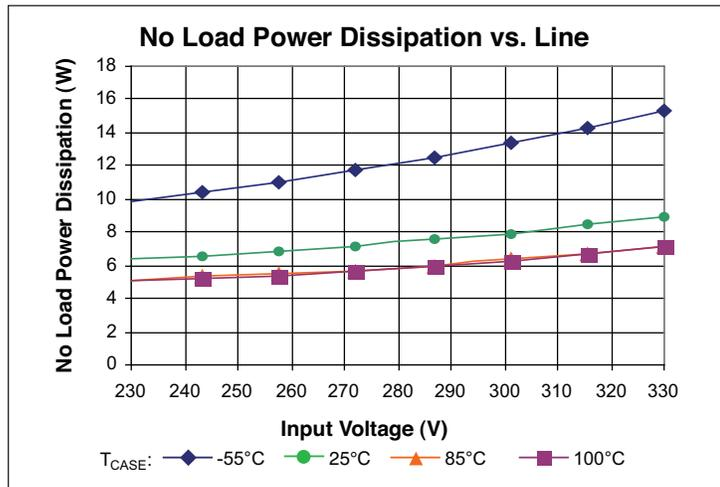
Figure 2 – No load power dissipation vs.  $V_{IN}$
