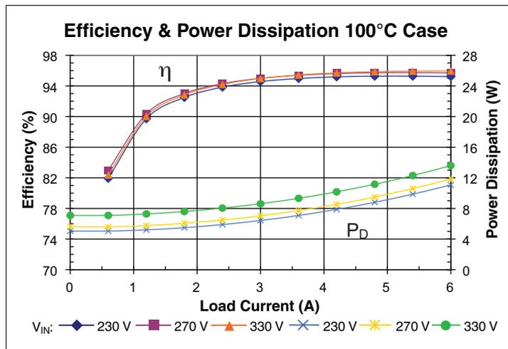
Figure 7 – Efficiency and power dissipation at  $T_C = 100^\circ\text{C}$
