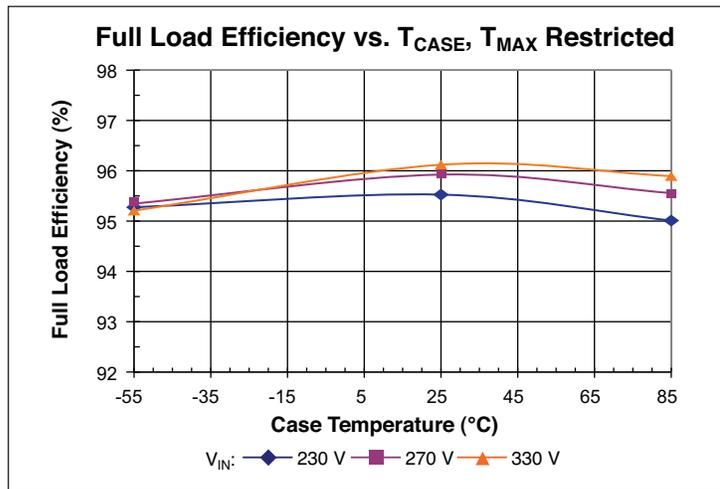
Figure 4 – Full load efficiency vs.  $T_{MAX}$  restricted
