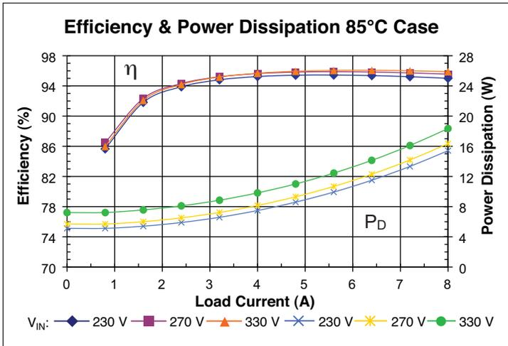
Figure 8 – Efficiency and power dissipation at  $T_C = 85^\circ\text{C}$
