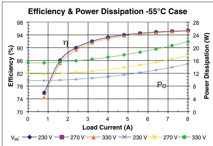
Figure 5 – Efficiency and power dissipation at  $T_C = -55^\circ\text{C}$
