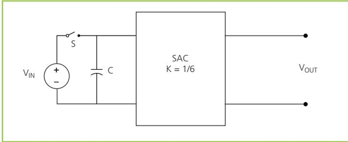
**Figure 16** – Sine Amplitude Converter™ with input capacitor
