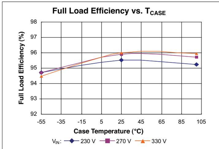
Figure 3 – Full load efficiency vs. full  $T_{MAX}$  range
