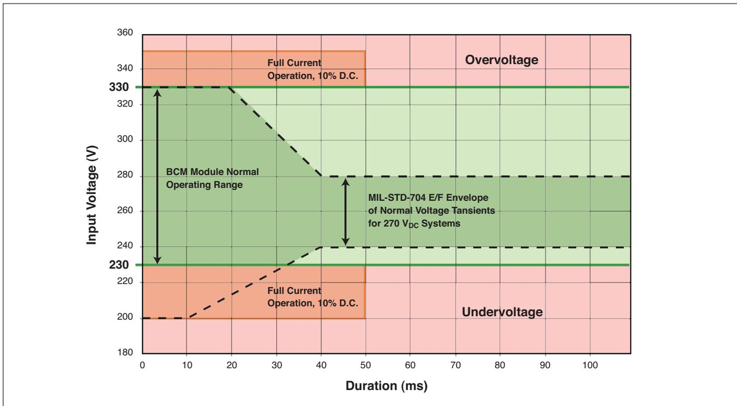
Figure 15 — Envelope of normal voltage transient for 270 V<sub>DC</sub> system.
