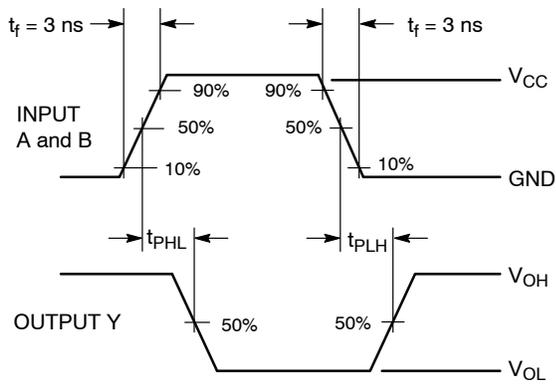
Figure 3. Switching Waveform
