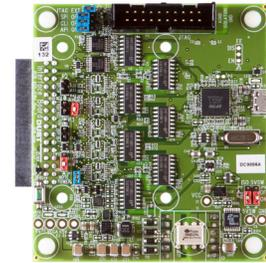
When connected to a DC9018A-B Evaluation/Development Mote, the **DC9006 Eterna interface card** provides a USB connection for both power and software access to the mote API UART port. The DC9006 comes with a DC9004 adapter card (not pictured) enabling the DC9006 to connect to the 10-pin programming and CLI header recommended for customer designs. Please see [www.linear.com/solutions/3102](http://www.linear.com/solutions/3102) for more details.
