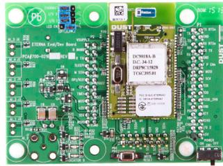
**SmartMesh IP Networks** are populated by motes, the nodes on the network. Based on the Dust® breakthrough Eterna® technology, the motes are ultralow power, extending battery life to years and many times that of alternative products. In addition to extra long battery life, the motes feature an advanced array of features.
