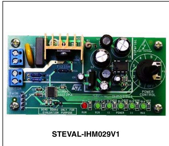
The power supply circuitry is based on the VIPer16L, an off-line converter with an 800 V avalanche-rugged power section, operating at 60 kHz.
