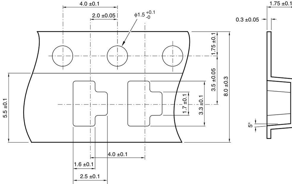
**Fig. 6 Reel Shape and Dimension**
