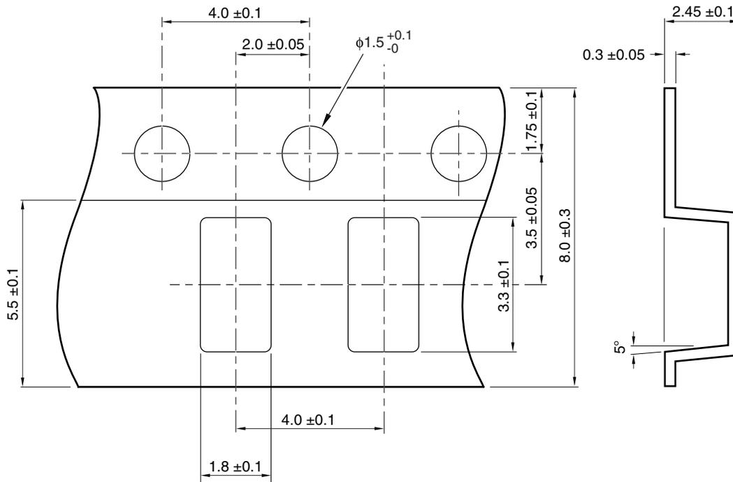
Fig. 9 Reel Shape and Dimension
