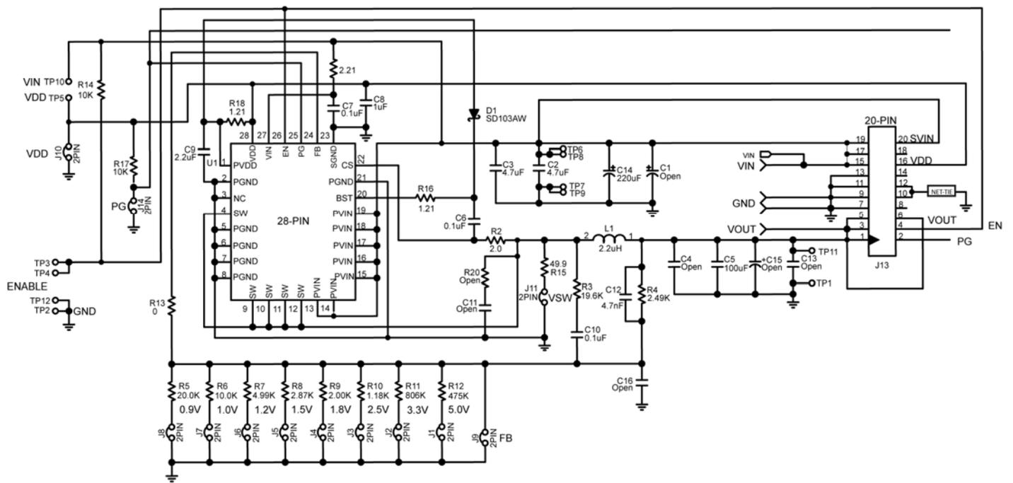
**Schematic of MIC26601 Evaluation Board
