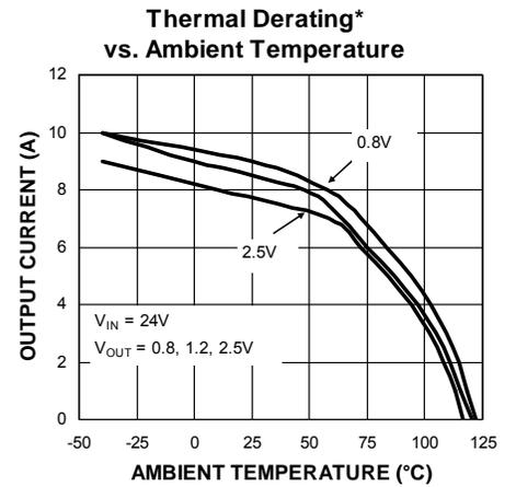
**Die Temperature\*** : The temperature measurement was taken at the hottest point on the MIC26601 case mounted on a 5 square inch 4 layer, 0.62", FR-4 PCB with 2oz finish copper weight per layer, see Thermal Measurement section. Actual results will depend upon the size of the PCB, ambient temperature and proximity to other heat emitting components.
