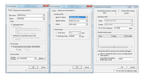
The flash memory write program is then downloaded to the microcontroller. The Output window in HEW will state 'Connected'.
