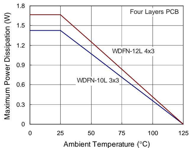
Figure 1. Derating Curves for RT9709/A Package
