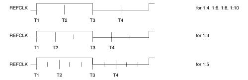
Figure 2-5. Internal Tick Spacing for Memory Controller Signals
