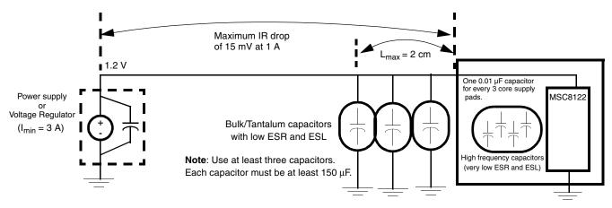
Figure 4-1. Core Power Supply Decoupling
