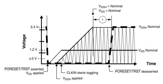
Figure 2-3. Start-Up Sequence with V<sub>DD</sub> Raised Before V<sub>DDH</sub> with CLKIN Started with V<sub>DDH</sub>
