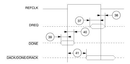
Figure 2-8. DMA Signals
