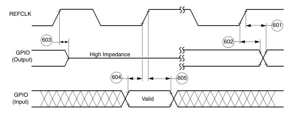
Figure 2-22. GPIO Timing
