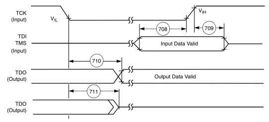
Figure 2-26. Test Access Port Timing Diagram
