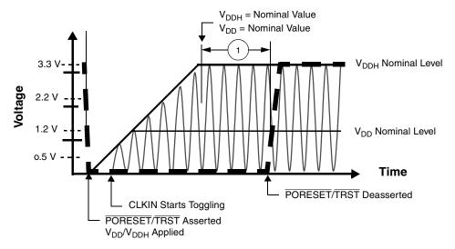
**Figure 2-2.** Start-Up Sequence with V<sub>DD</sub> and V<sub>DDH</sub> Raised Together
