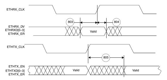
Figure 2-19. MII Mode Signal Timing
