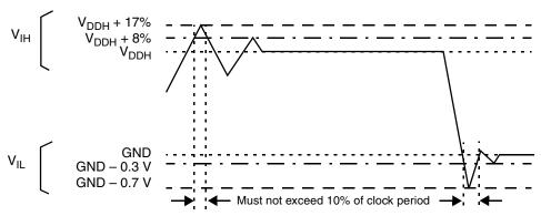
Figure 2-1. Overshoot/Undershoot Voltage for V<sub>IH</sub> and V<sub>IL</sub>
