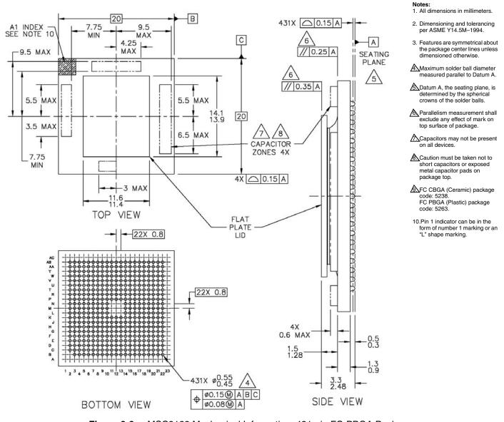
Figure 3-3. MSC8122 Mechanical Information, 431-pin FC-PBGA Package
