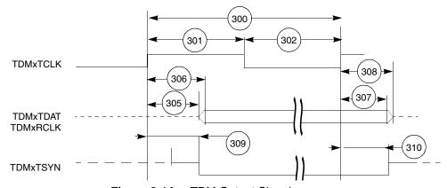
Figure 2-14. TDM Output Signals
