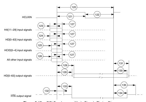
Figure 2-12. DSI Synchronous Mode Signals Timing Diagram
