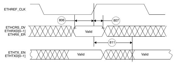
Figure 2-20. RMII Mode Signal Timing
