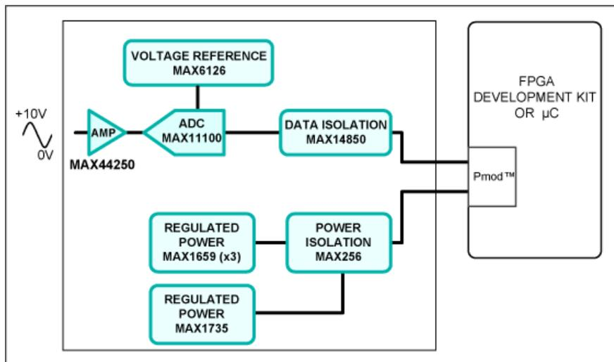
Figure 1. The Fresno subsystem design block diagram.
