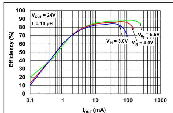
**FIGURE 2-6:** 24.0V  $V_{OUT}$  Efficiency vs.  $I_{OUT}$ .
