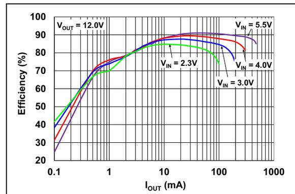
**FIGURE 2-5:** 12.0V  $V_{OUT}$  Efficiency vs.  $I_{OUT}$ .
