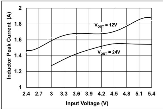
**FIGURE 2-7:** Inductor Peak Current Limit vs. Input Voltage.
