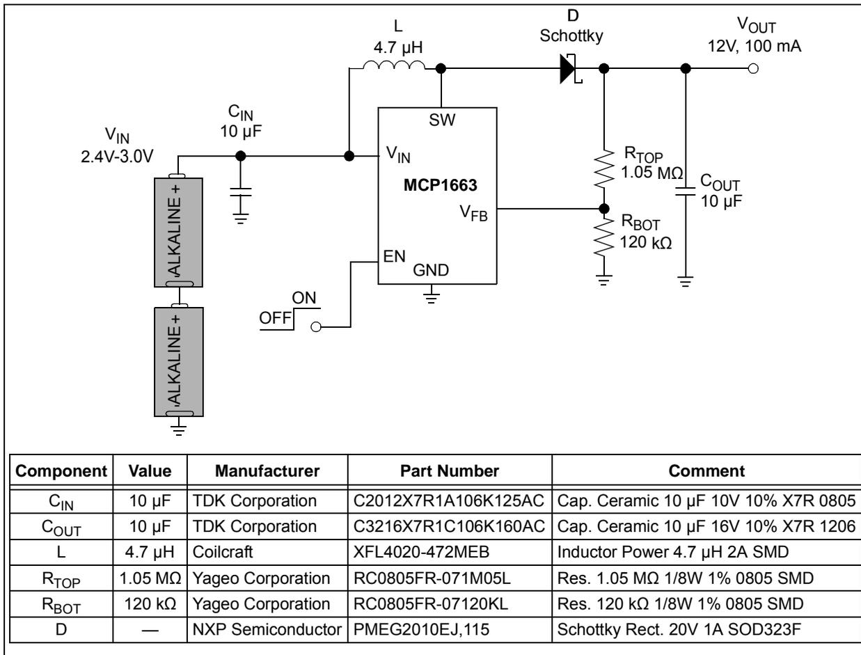
**FIGURE 6-1:** Two Alkaline Cells to 12V Boost Converter.
