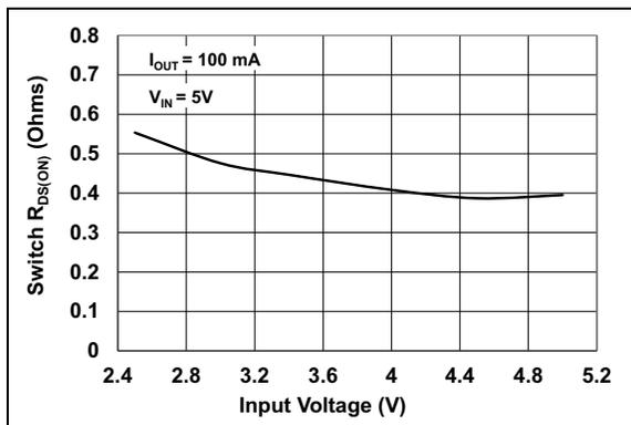
**FIGURE 2-14:** N-Channel Switch  $R_{DS(on)}$  vs.  $V_{IN}$ .
