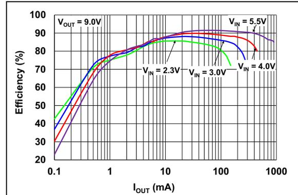
**FIGURE 2-4:** 9.0V  $V_{OUT}$  Efficiency vs.  $I_{OUT}$ .
