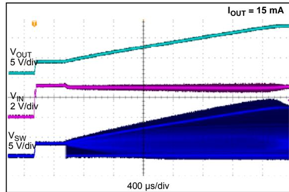
**FIGURE 2-18:** 12.0V Start-Up ( $V_{IN} = V_{ENABLE}$ ).
