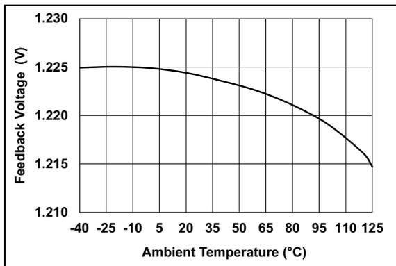
**FIGURE 2-2:**  $V_{FB}$  Voltage vs. Ambient Temperature and  $V_{IN}$ .
