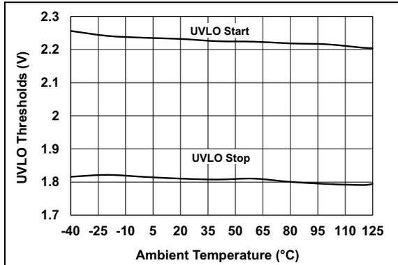
**FIGURE 2-1:** Undervoltage Lockout (UVLO) vs. Ambient Temperature.
