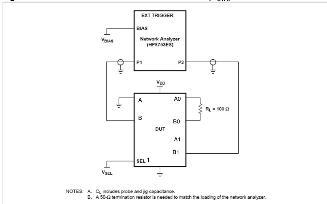
Off isolation is measured at the output of the OFF channel. For example, when  $V_{SEL1}=0$ , and B is the input, the output is measured at B1. All unused analog input ports are connected to GND and output ports are left open.
