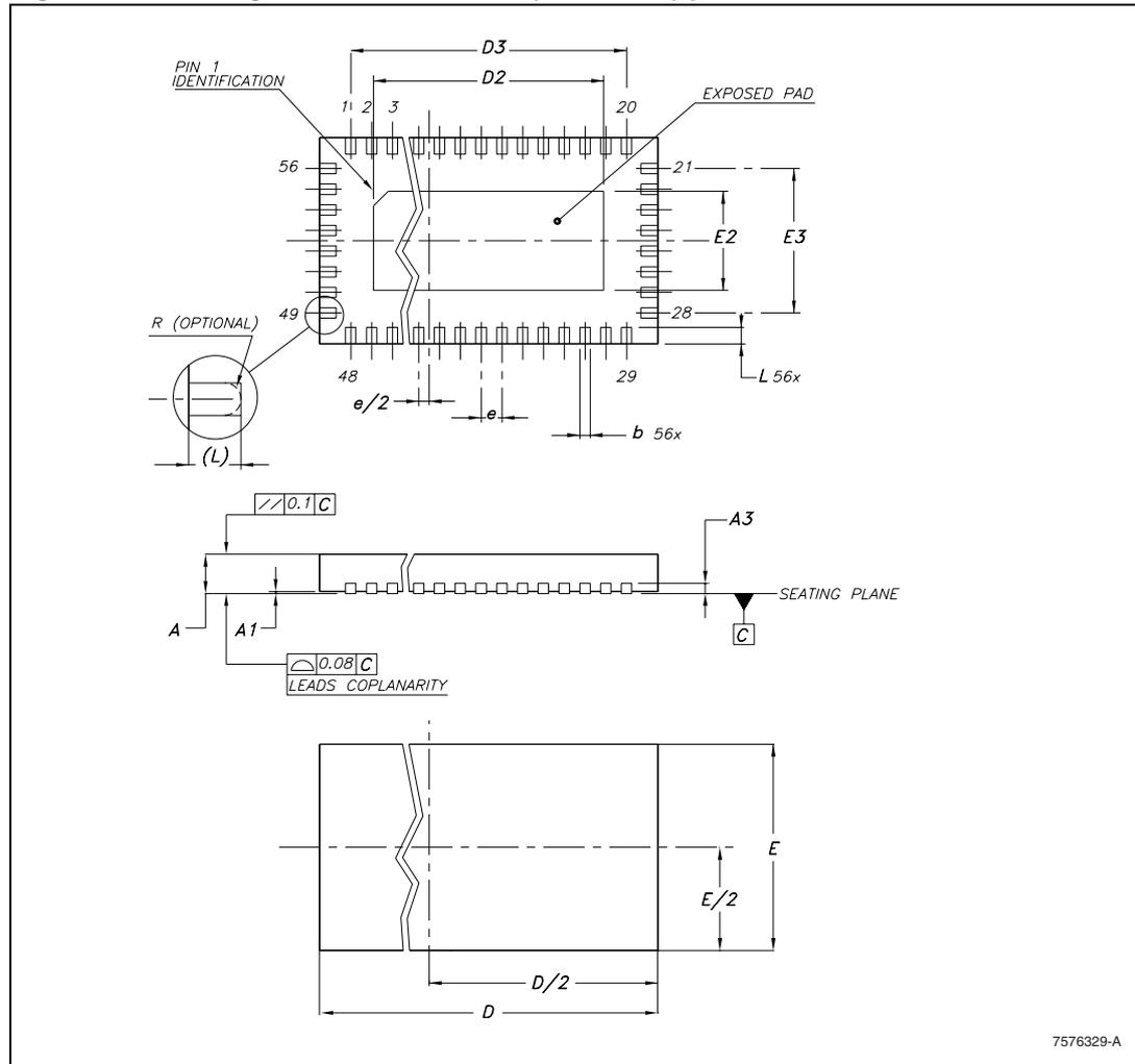
Table 13. Mechanical data for QFN56 (11 x 5 mm) pitch 0.5 mm
