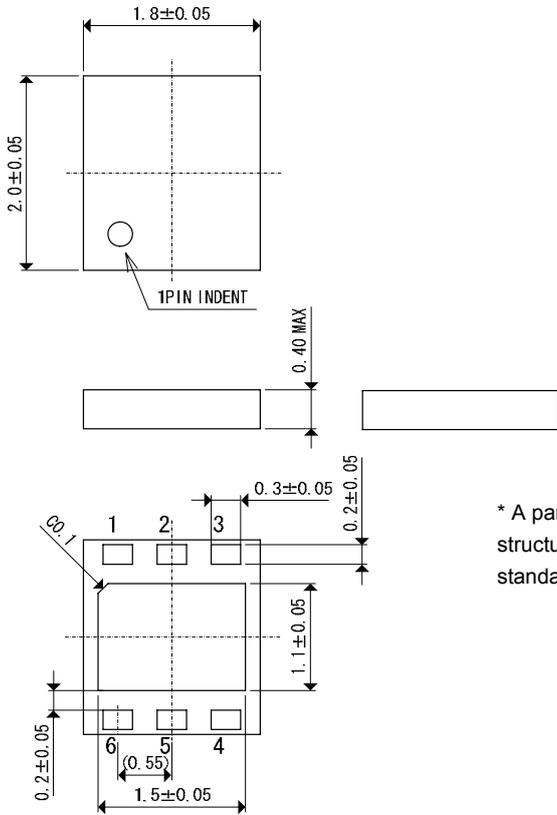
\* A part of the pin may appear from the side of the package because of it's structure, but reliability of the package and strength will not be changed below the standard.
