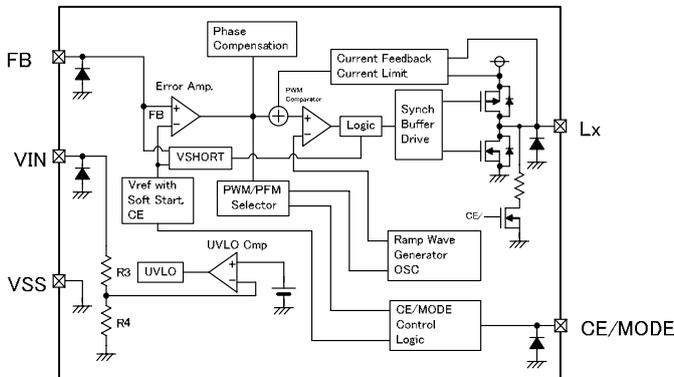
NOTE: The signal from CE/MODE Control Logic to PWM/PFM Selector is being fixed to "L" level inside, and XC9235 series chooses only PWM control.
