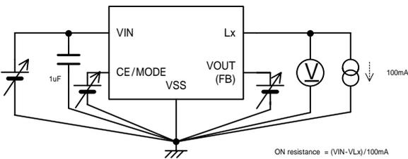
$$\text{ON resistance} = (V_{in} - V_{Lx}) / 100\text{mA}$$
