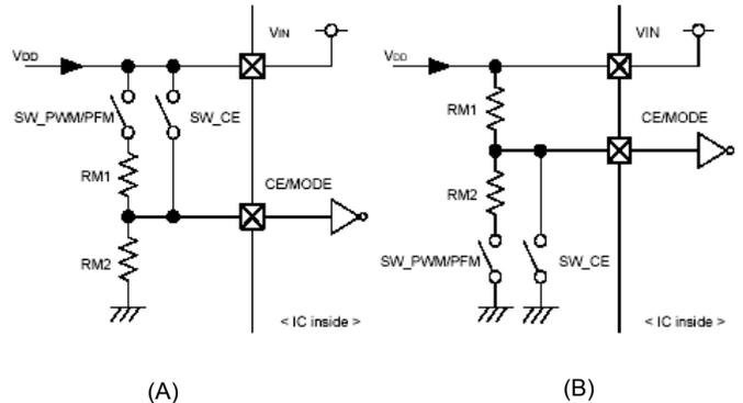
Intermediate voltage can be generated by RM1 and RM2. Please set the value of each R1, R2, RM1, RM2 from few hundreds k to few hundreds M. For switches, CPU open-drain I/O port and transistor can be used.
