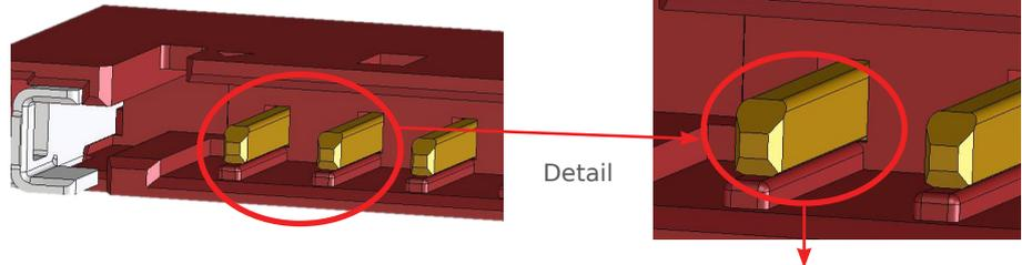
Header pins have a beveled shape and are set back on housing ridge to provide mating guidance and protection. (1.00mm pitch version shown)
