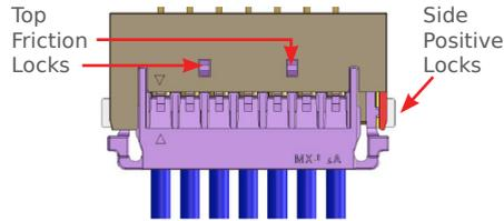
Side positive locks provide secure mating retention and space savings compared to top-style locks. (1.50mm pitch version shown)
