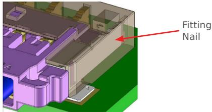
Fitting nails wrap around the header and housing to provide secure PCB retention support and added mechanical stability. (1.50mm pitch version shown)
