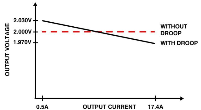
**FIGURE 4. OUTPUT VOLTAGE DROOP AT 2.0V DAC SETTING**
