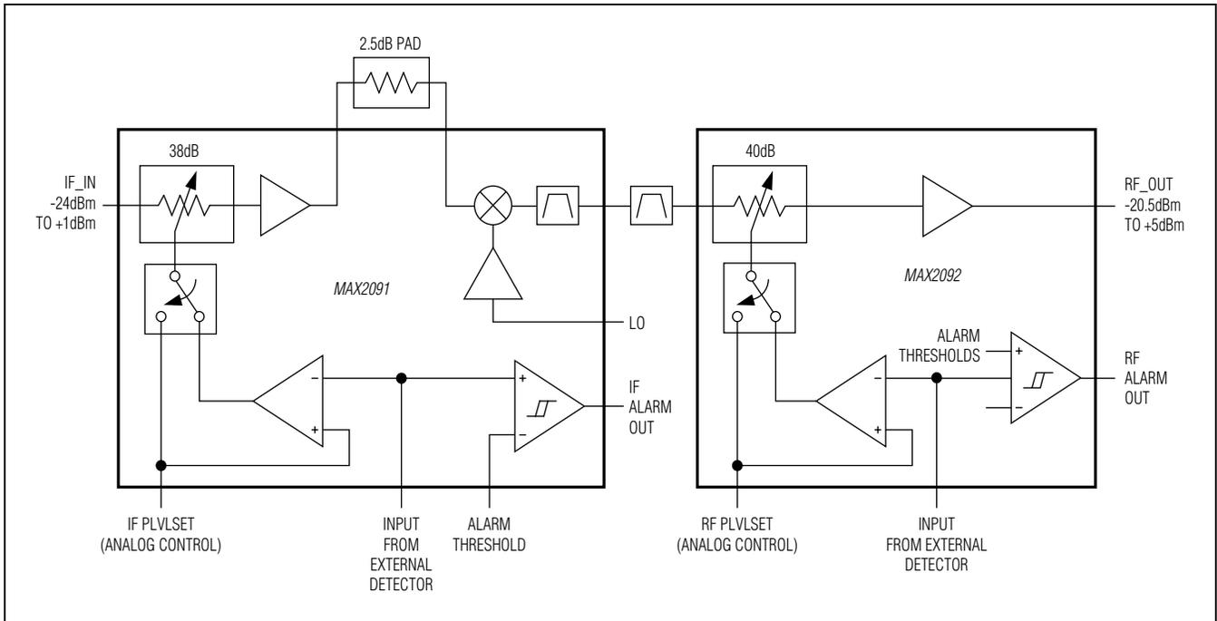
Figure 1. Cascaded IF-RF Lineup Using the MAX2091 + MAX2092
