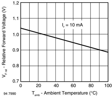
Fig. 5 - Relative Forward Voltage vs. Ambient Temperature
