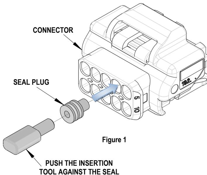
2. Gently push the Seal Plug with the insertion tool into the desired cavity of the connector until it stops.
