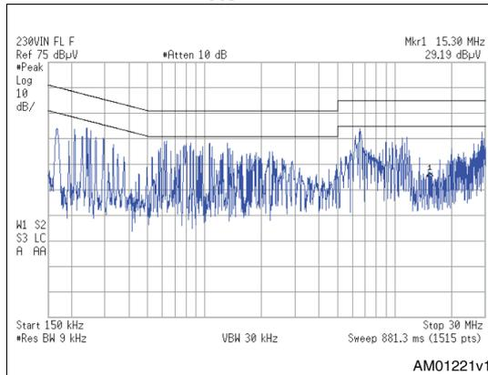
Figure 25. 230 V<sub>AC</sub> and full load - neutral
