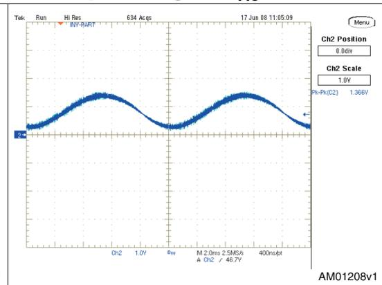
In [Figure 10](#) and [Figure 11](#) the output voltage ripple at twice the input mains frequency is measured. As shown it is less than 0.4 V peak-to-peak, which is ideal for LED or lighting applications. High frequency noise, including spikes, is significantly reduced as well.
