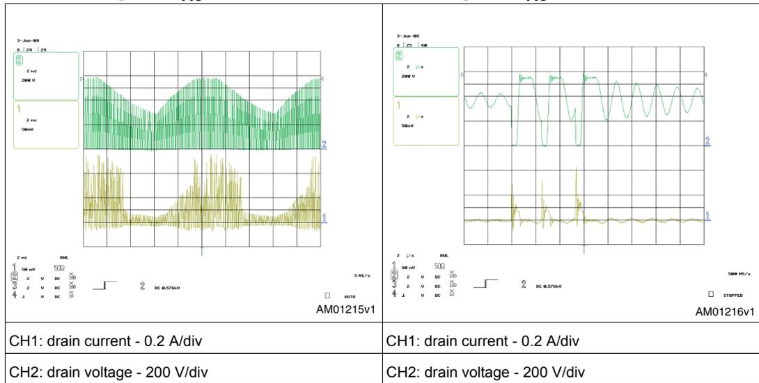
The above figures show the MOSFET waveforms at light load. Even in this load condition the waveforms are correct. It can be noted that at high mains the converter works in burst mode (see [Figure 19](#)), keeping efficiency at a good level.
