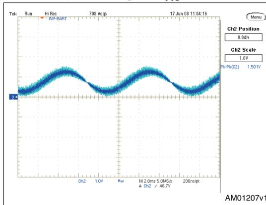
Figure 11. EVL6562A-35WFLB output voltage ripple @ 265 V<sub>AC</sub> - full load
