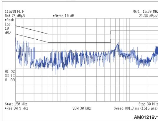
Figure 23. 115 V<sub>AC</sub> and full load - neutral
