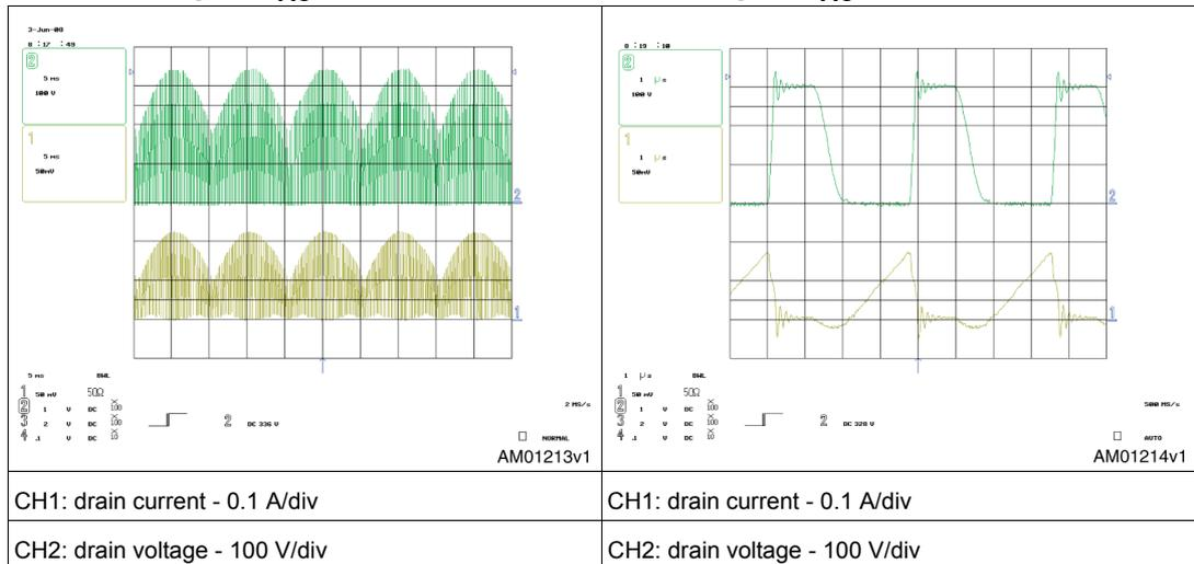
**Figure 18. EVL6562A-35WFLB  $V_{DS}$  and  $I_D$  @ 265  $V_{AC}$  - 40 mA**      **Figure 19. EVL6562A-35WFLB  $V_{DS}$  and  $I_D$  @ 265  $V_{AC}$  - 40 mA - detail**
