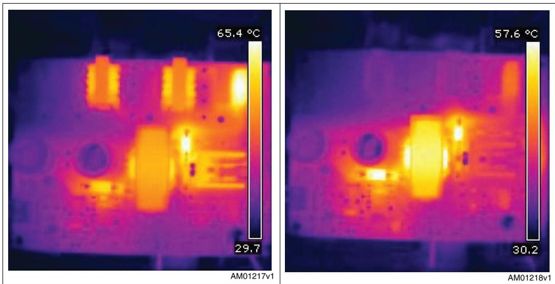
**Table 2. Measured temperature @ 90 V<sub>AC</sub> and 265 V<sub>AC</sub> - full load**
