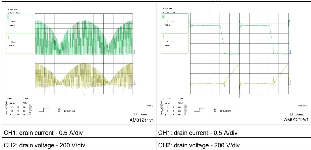
Figure 14 shows the measurement at the maximum drain voltage of 265  $V_{AC}$  and max load. In this worst-case condition, the peak drain voltage is 640  $V_{PK}$ , assuring a good margin with respect to the MOSFET  $BV_{DSS}$  and contributing strongly to the reliability and low failure rate of the design.
