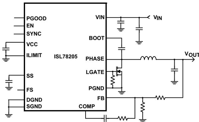
FIGURE 1. TYPICAL APPLICATION SCHEMATIC I - SYNCHRONOUS BUCK
