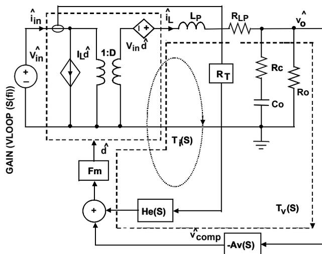
FIGURE 18. SMALL SIGNAL MODEL OF BUCK REGULATOR
