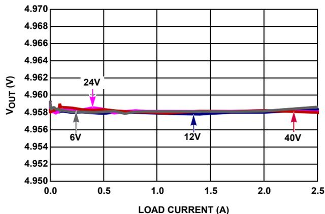
FIGURE 5. LOAD REGULATION,  $V_{OUT}$  5V,  $T_A = +25^\circ\text{C}$
