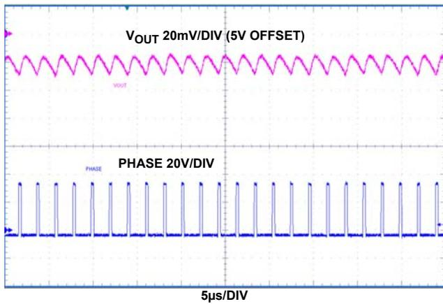
FIGURE 11. SYNCHRONOUS BUCK,  $V_{IN}$  36V,  $I_O$  2A
