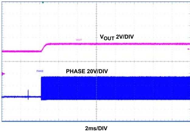
FIGURE 9.  $V_{IN}$  36V, PRE-BIASED START-UP
