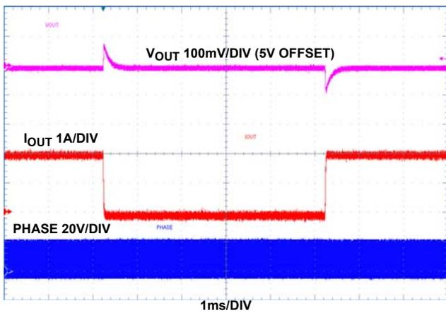
FIGURE 13.  $V_{IN}$  24V, 0A TO 2A STEP LOAD
