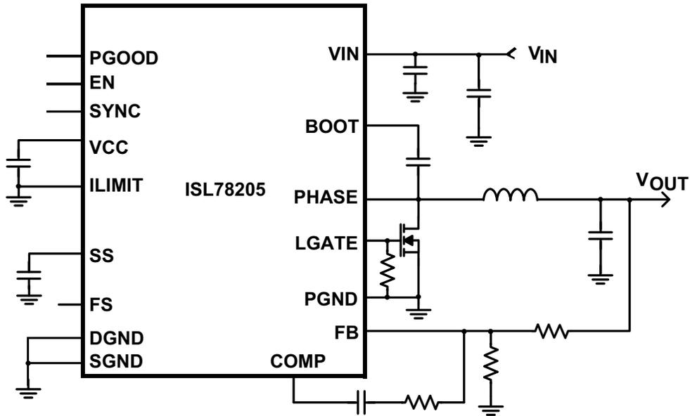
**Typical Application Schematic II - Non-Synchronous Buck**
