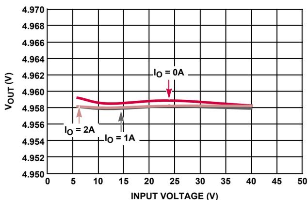
FIGURE 6. LINE REGULATION,  $V_{OUT}$  5V,  $T_A = +25^\circ\text{C}$
