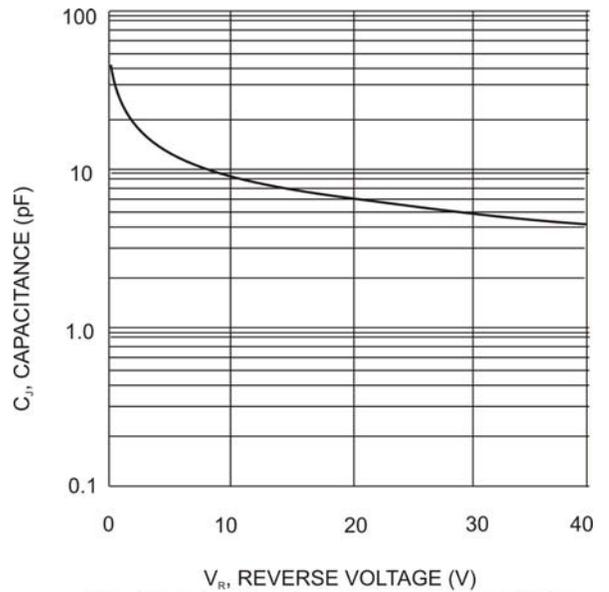
Fig. 4 Typ. Junction Capacitance vs Reverse Voltage
